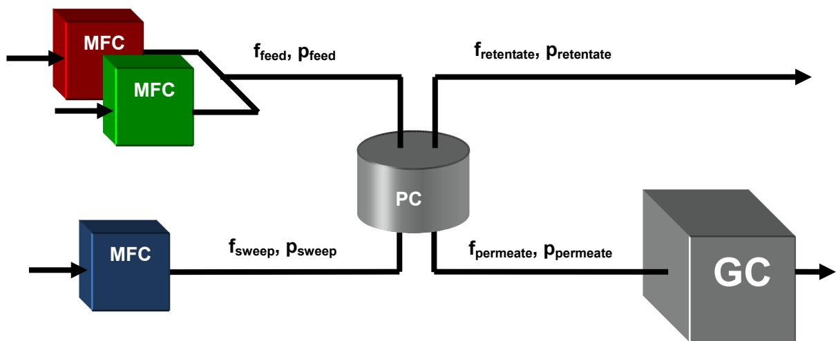
**Figure S8.** Measurement equipment for both single and mixed gas permeation.
