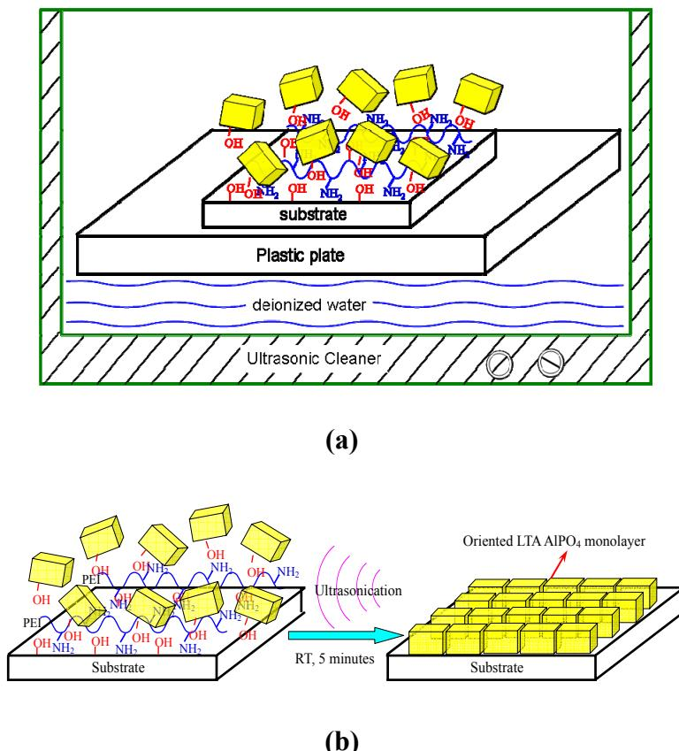
**Figure S1.** Scheme for the sonication set up (a) and the assembling of AlPO<sub>4</sub> LTA microcrystals by ultrasonication using polyethylenimine (PEI) as mediator between the AlPO<sub>4</sub> LTA crystals thus forming a highly oriented seed crystal monolayer (b).
