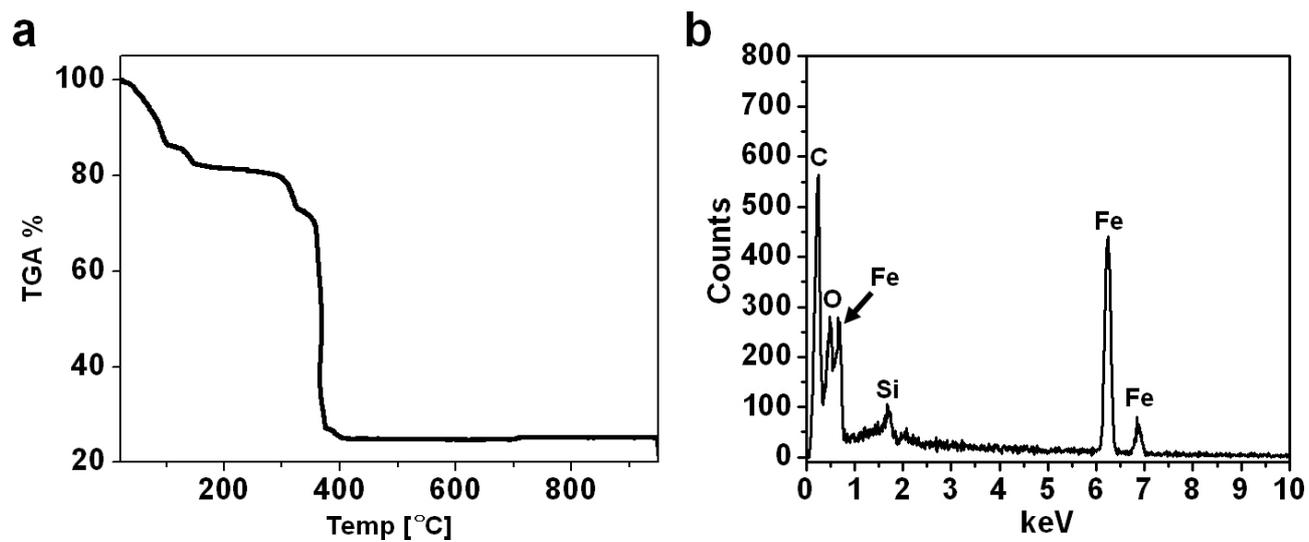
**Fig. S1** (a) TGA curve and (b) EDX spectrum of coordination polymer nanorods (CPP-15).
