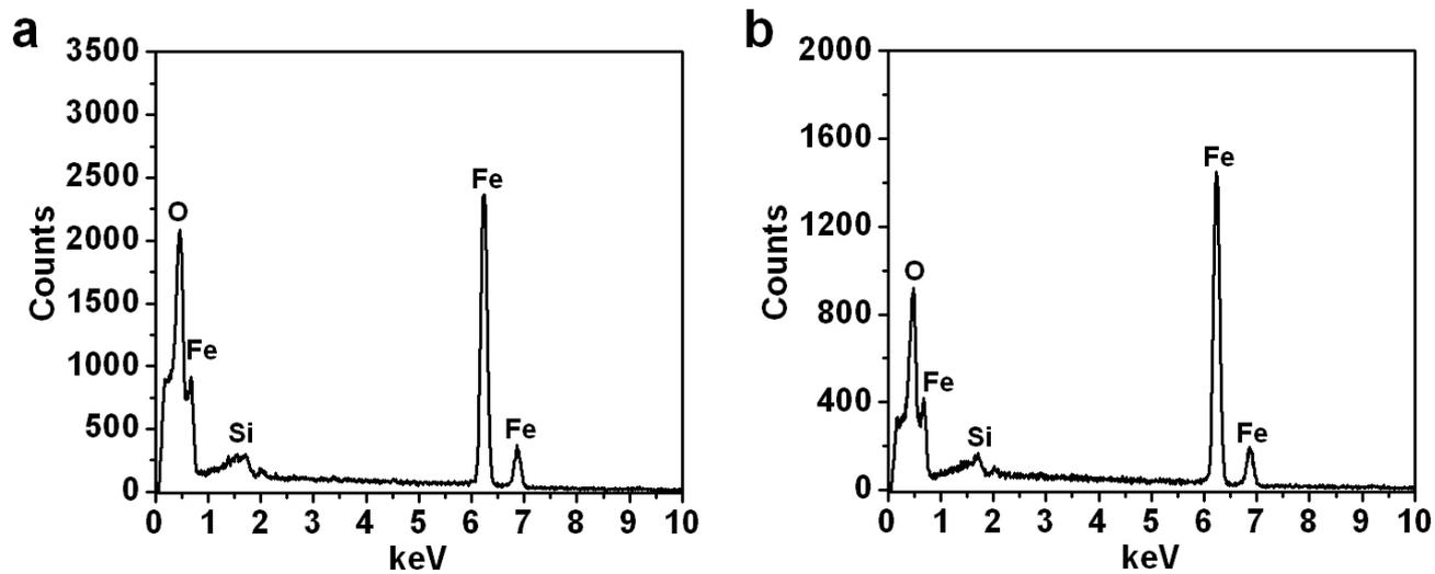
Fig. S4 EDX spectra of (a) hematite ( $\alpha\text{-Fe}_2\text{O}_3$ ) nanorods and (b) magnetite ( $\text{Fe}_3\text{O}_4$ ) nanorods.
