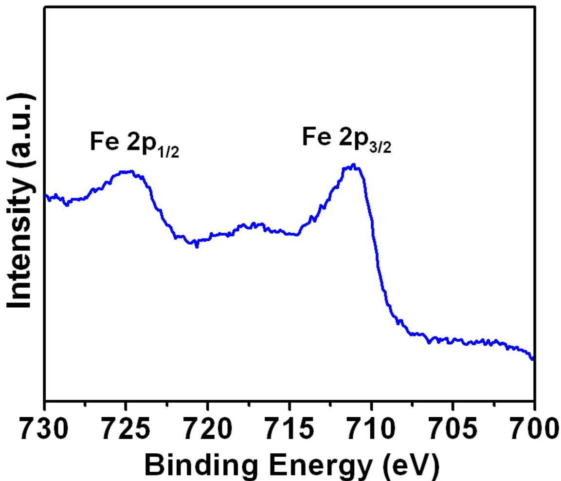
**Fig. S3** XPS data of CPP-15. The binding energies of Fe2p<sub>3/2</sub> (711.1 eV) and Fe2p<sub>1/2</sub> (724.6 eV) are close to the reported values observed for Fe(III) compounds.
