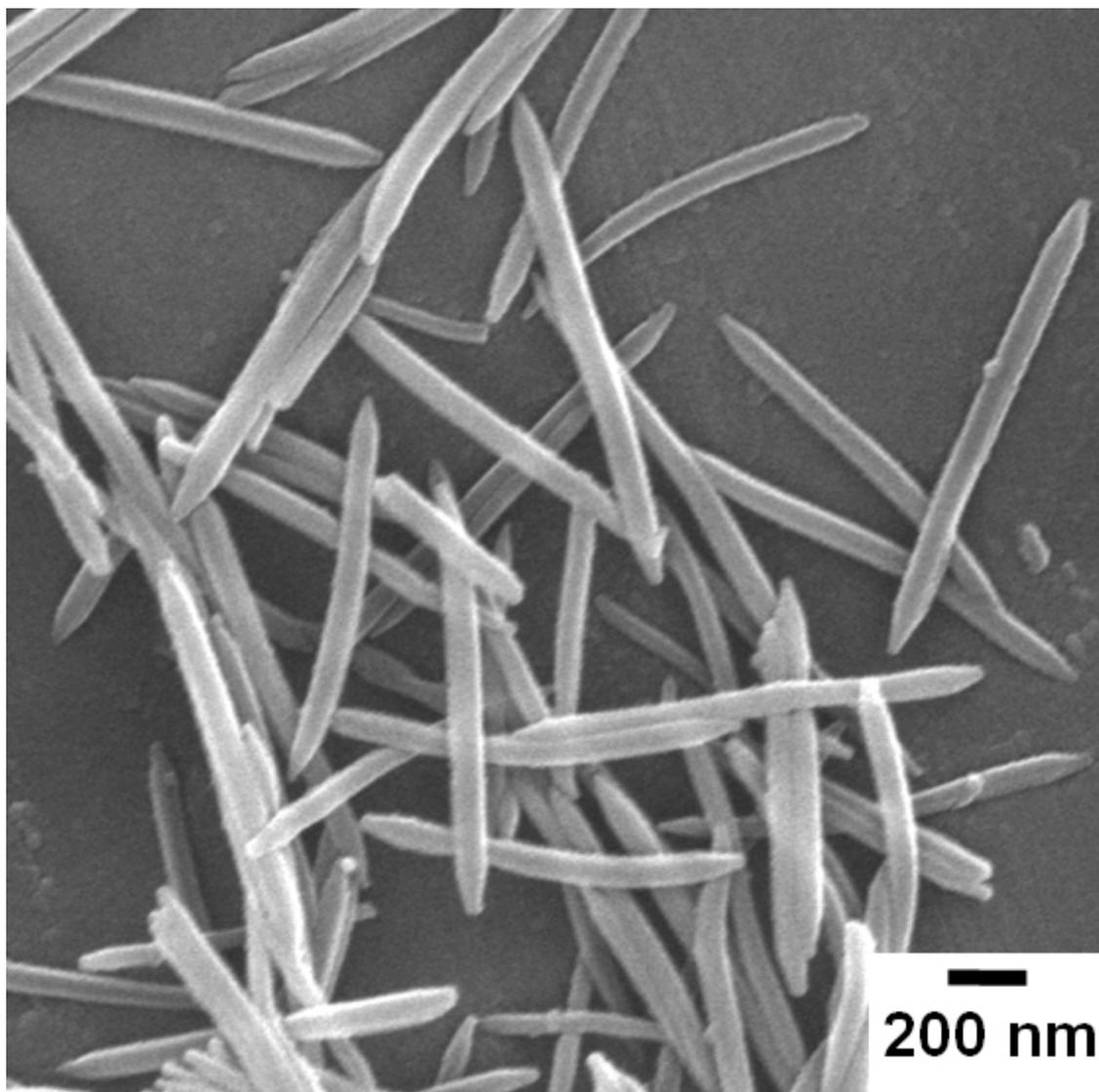
**Fig. S5** SEM image of hematite nanorods containing the organic residues prepared by incomplete calcination at 300 °C in air for 50 min.
