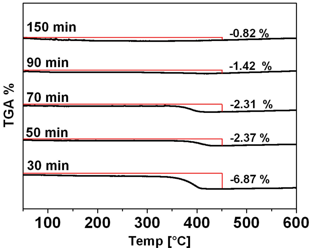
**Fig. S6** TGA curves of hematite nanorods containing the organic residues prepared by incomplete calcination at 300 °C in air for 30, 50, 70, 90 and 150 min. These show the approximate amount of organic residues within the incompletely calcined particles.
