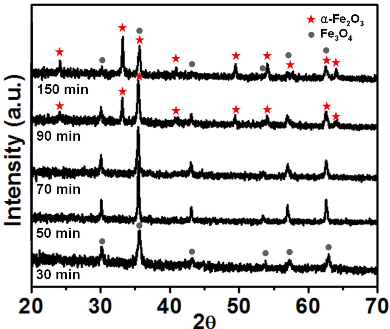
Fig. S7 PXR D patterns of final products after the second thermal treatment at 700 °C under  $\text{N}_2$  atmosphere on a series of the incompletely calcined particles containing the organic residues prepared by incomplete calcination at 300 °C in air for 30, 50, 70, 90 and 150 min. There was no complete phase transformation in the samples containing small amount of organic residues as a result of long holding time (90 and 150 min) during the first thermal treatment.
