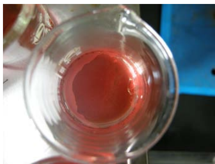
Fig. S1. Image of 18-nm AuNP monolayer film obtained by injecting the mixture with the ethanol:toluene volume ratio of 1:3 from the bottom of a 25-mL beaker (inner diameter, 3.5 cm) containing AuNP solution. The injected volume of ethanol was fixed at 2.75 mL.
