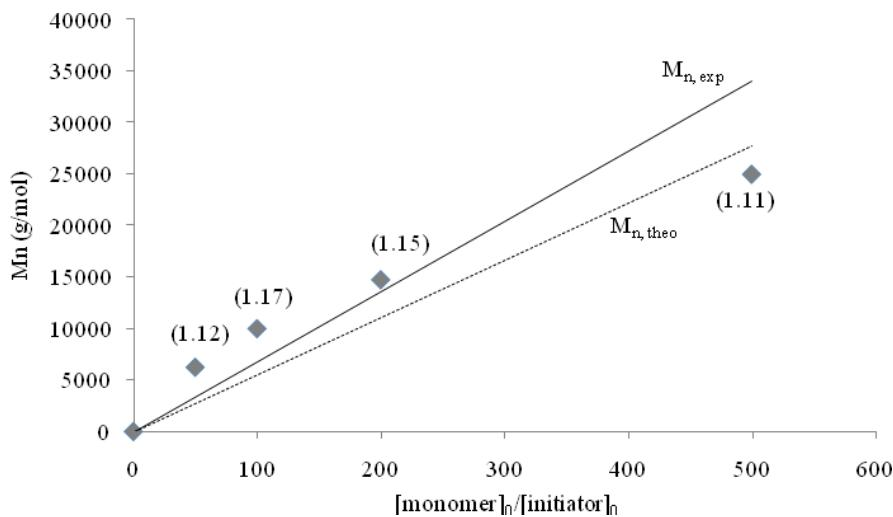
**Figure S2** Polymerization of *meso*-lactide by **5** in toluene, Initial ratio variation, T = 100 °C.
