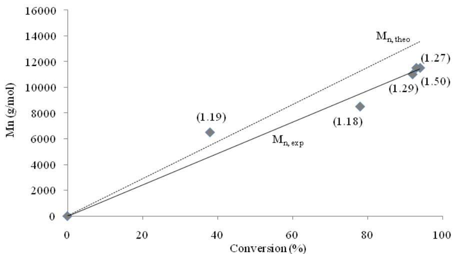
**Figure S4** Polymerization of *L*-lactide by **5** in toluene, [monomer]/[initiator] = 100, T = 100 °C.
