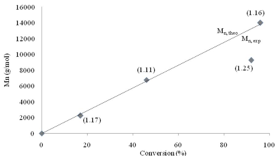
**Figure S3** Polymerization of *rac*-lactide by 5 in toluene, [monomer]/[initiator] = 100, T = 100 °C.
