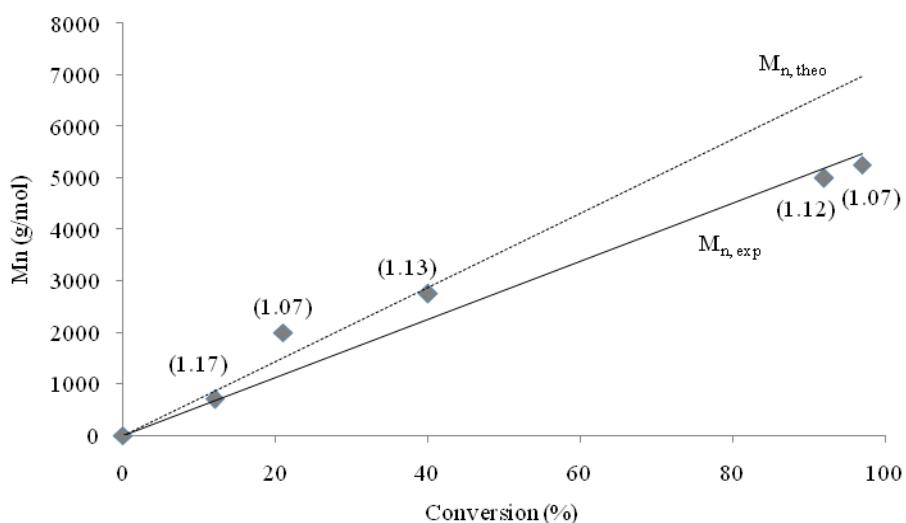
**Figure S1** Polymerization of *meso*-lactide by **5** in toluene, [monomer]/[initiator] = 100,  $T=75$  °C.
