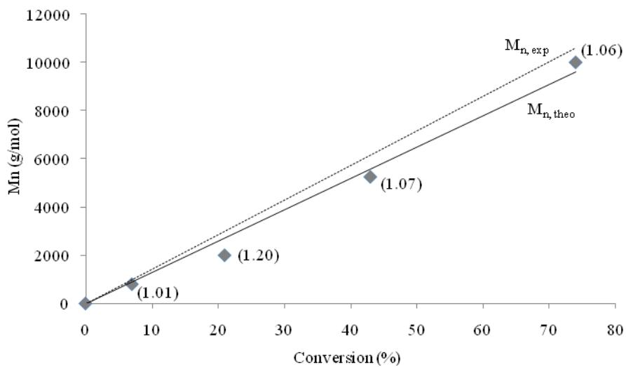
**Figure S5** Polymerization of *meso*-lactide by **5** in melt, [monomer]/[initiator] = 100, T = 100 °C.
