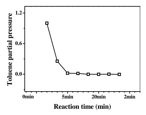
$TiO_2/AAO$  (300 cycles) was used for toluene adsorption experiment. Initially toluene partial pressure in th e chamber was 5 mtorr, and whereas that of  $N_2$  80 mtorr.  $O_2$  partial pressure was 20 mtorr. Toluene can c ompletely be removed within 5 minutes
