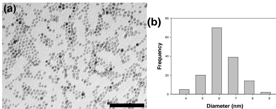
**Fig. S3.** (a) TEM image and (b) size histogram of as-synthesized iron oxide nanocrystals. Scale bar represent 200 nm.
