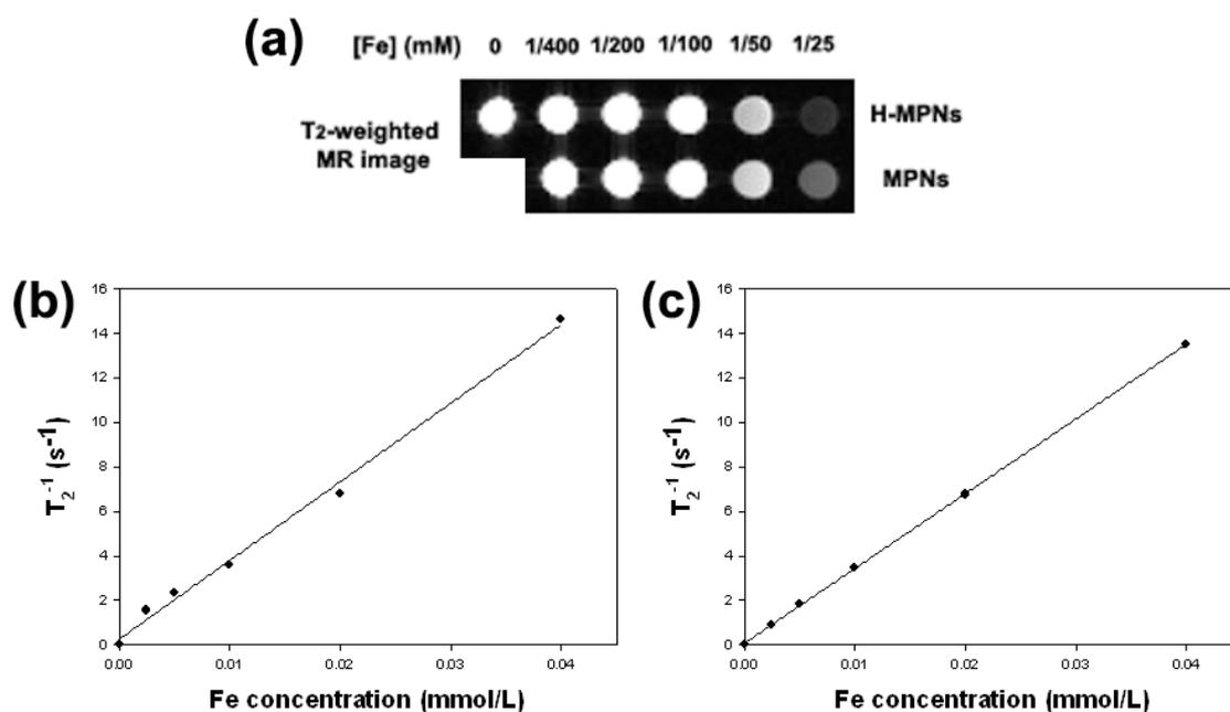
**Fig. S7** (a) T<sub>2</sub>-weighted MR images of H-MPNs and MPNs in aqueous solution with various concentrations at 4.7 T. (b) graph of R<sub>2</sub> against the iron concentration in H-MPNs. (c) graph of R<sub>2</sub> against the iron concentration in MPNs.
