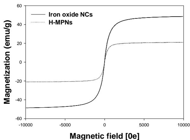
**Fig. S6.** Magnetization curves of iron oxide nanocrystals and H-MPNs at room temperature.
