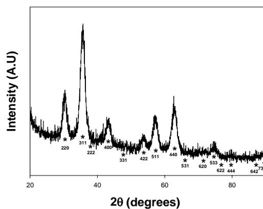
**Fig. S4.** X-ray diffraction patterns of 6 nm sized iron oxide nanocrystals.
