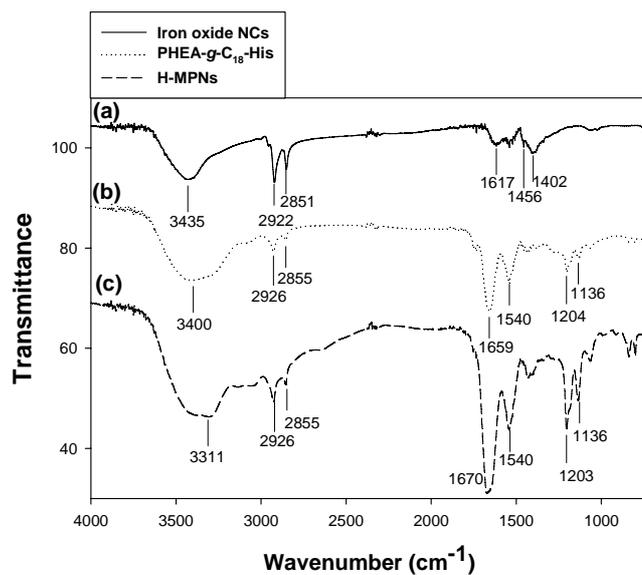
**Fig. S5.** FT-IR spectra of (a) 6 nm sized iron oxide nanocrystals, (b) PHEA-g-C<sub>18</sub>-His and (c) H-MPNs.
