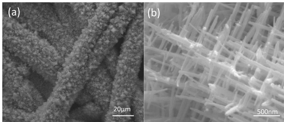
**Figure S2** (a) Low-magnification and (b) High-magnification SEM images of 3D  $\text{WO}_3$  nanostructures after dye degradation experiments.
