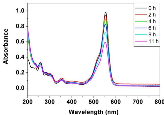
**Figure S1** UV-vis absorption spectra of RB solution as a function of irradiation time with the absence of 3D  $\text{WO}_3$  nanostructures on carbon paper.
