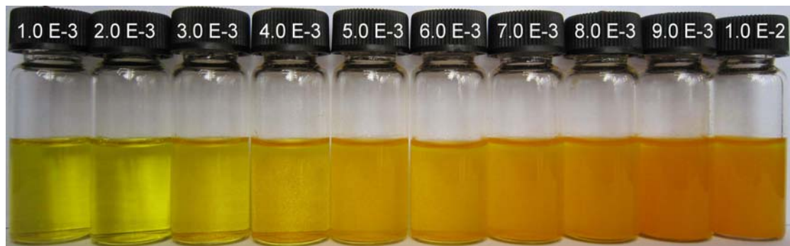
Fig. S3 The image of L ( 9.0 \times 10^{-4} M) with TNP ( 1.0 \times 10^{-3} – 1.0 \times 10^{-2} M) in ethanol (0.5% DMF, v/v).
