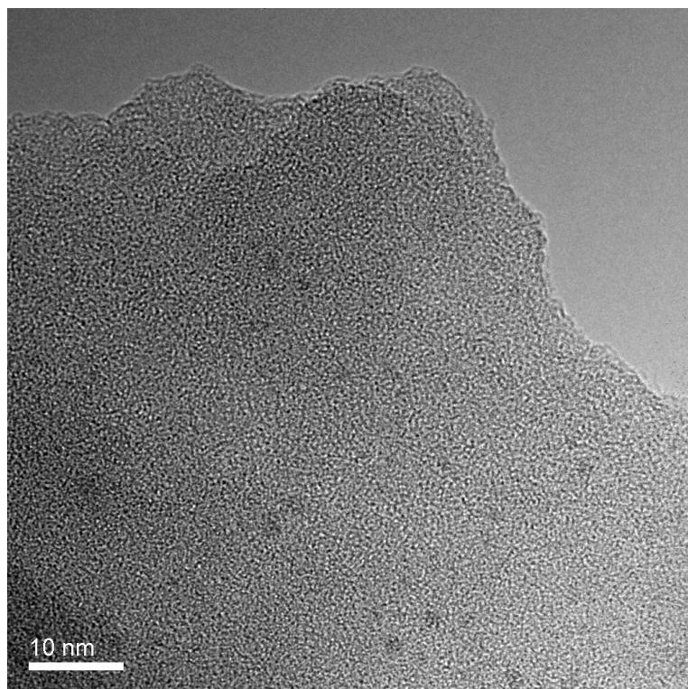
**Figure S1** TEM image of graphene-Pd without phosphonated calix[4]arene.
