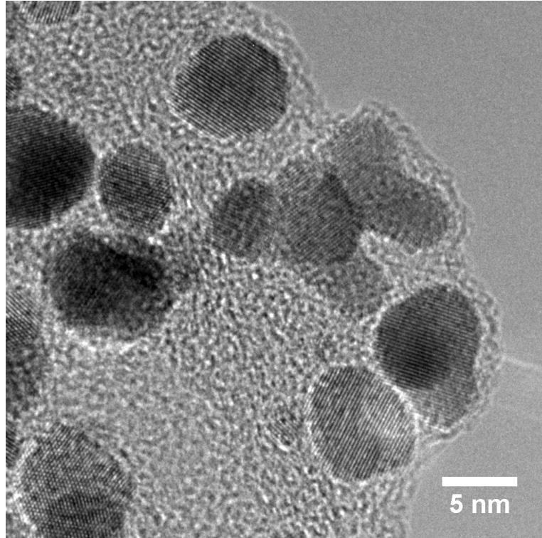
**Figure S3.** High resolution TEM image of Pt nanoparticles on the CSG.
