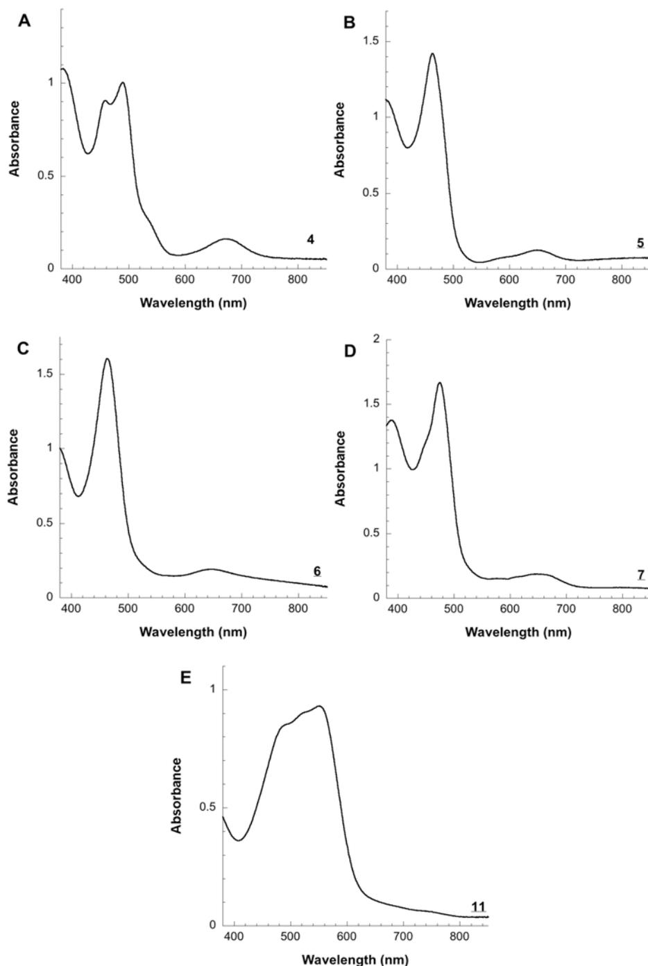
Figure S2. UV-Visible spectra of TAM-Nu **4** (A), **5** (B), **6** (C), **7** (D), and **11** (E) (in MeOH except for **11**: in CH<sub>2</sub>Cl<sub>2</sub>)
