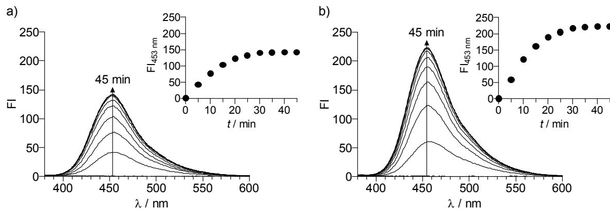
**Fig. S7** Time-dependent change in the fluorescence spectra ( $\lambda_{\text{ex}} = 309 \text{ nm}$ ) of **2** (10  $\mu\text{M}$ ) measured after addition of (a) 10 equiv or (b) 50 equiv of  $\text{CN}^-$  in a buffered water/MeCN mixture (8/2 v/v; CHES 100 mM, pH 9.3) under UV irradiation (334 nm) at 25  $^\circ\text{C}$ . (Inset) Change in fluorescence intensity at 453 nm.
