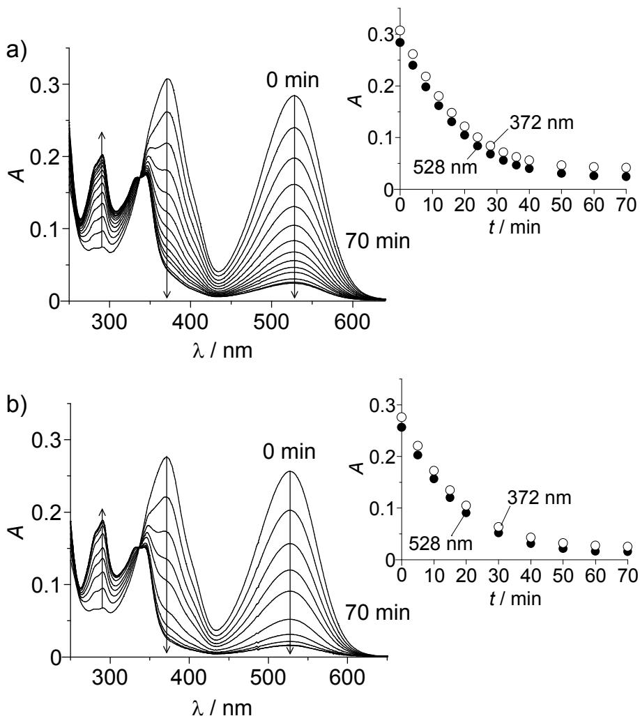
**Fig. S5** Time-dependent change in absorption spectra of **2** (10  $\mu$ M) measured in a buffered water/MeCN mixture (8/2 v/v; CHES 100 mM, pH 9.3) under irradiation of (a) 380 nm and (b) 550 nm monochrommatic light at 25 °C.
