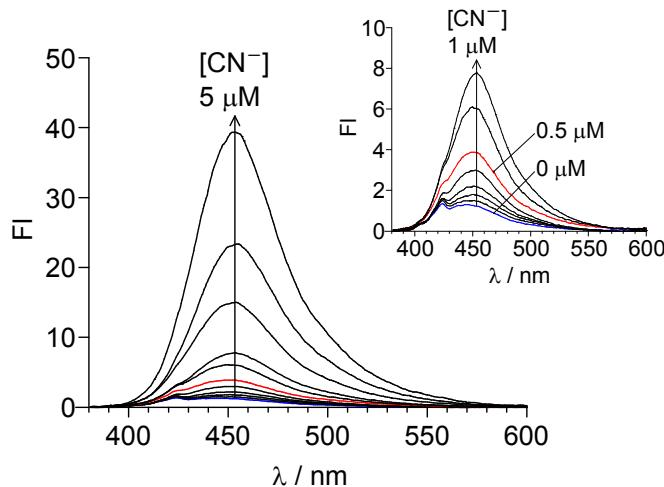
**Fig. S10** Change in fluorescence spectra ( $\lambda_{\text{ex}} = 372 \text{ nm}$ ) of **2** (10  $\mu\text{M}$ ) during titration with  $\text{CN}^-$  in a buffered water/MeCN mixture (8/2 v/v; CHES 100 mM, pH 9.3) under UV irradiation (334 nm) at 25 °C. The spectra at each  $\text{CN}^-$  concentration were obtained after stirring the solution for 30 min under UV irradiation. The blue and red spectra were obtained with 0 and 0.5  $\mu\text{M}$   $\text{CN}^-$ .
