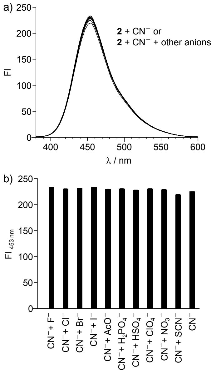
**Fig. S6** (a) Fluorescence spectra ( $\lambda_{\text{ex}} = 309 \text{ nm}$ ) of **2** (10  $\mu\text{M}$ ) measured with 50 equiv of  $\text{CN}^-$  together with 50 equiv of other respective anions in a buffered water/MeCN mixture (8/2 v/v; CHES 100 mM, pH 9.3) under UV irradiation (334 nm) at 25  $^{\circ}\text{C}$ . The fluorescence measurements were carried out after the solution was stirred for 30 min under UV irradiation. (b) Fluorescence intensity of the respective solutions.
