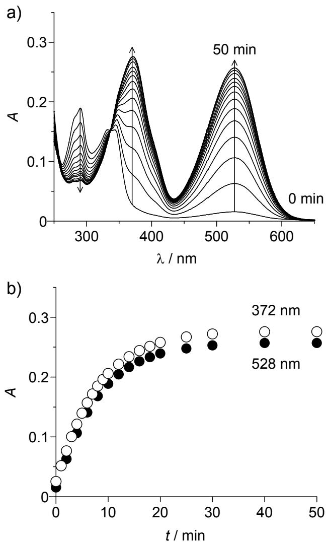
**Fig. S4** (a) Time-dependent change in absorption spectra of **2** (10  $\mu\text{M}$ ) measured in a buffered water/MeCN mixture (8/2 v/v; CHES 100 mM, pH 9.3) under UV irradiation (334 nm) at 25 °C. (b) Change in absorbance of 372 and 528 nm bands.
