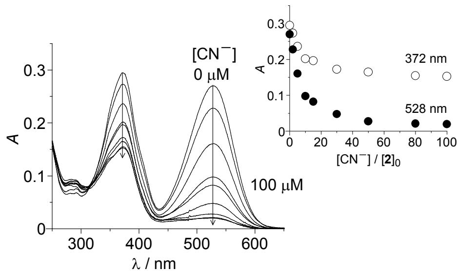
**Fig. S8** Absorption titration of **2** (10  $\mu\text{M}$ ) with  $\text{CN}^-$  in a buffered water/MeCN mixture (8/2 v/v; CHES 100 mM, pH 9.3) under UV irradiation (334 nm) at 25  $^\circ\text{C}$ . Each spectrum was obtained after stirring the solution for 30 min with UV irradiation. (Inset) Change in absorbance of 372 and 528 nm bands.
