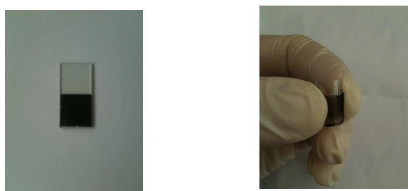
Figure S2. Transferred and vertically oriented N-CNTs on ITO/Glass (left) and on ITO/PEN (right).
