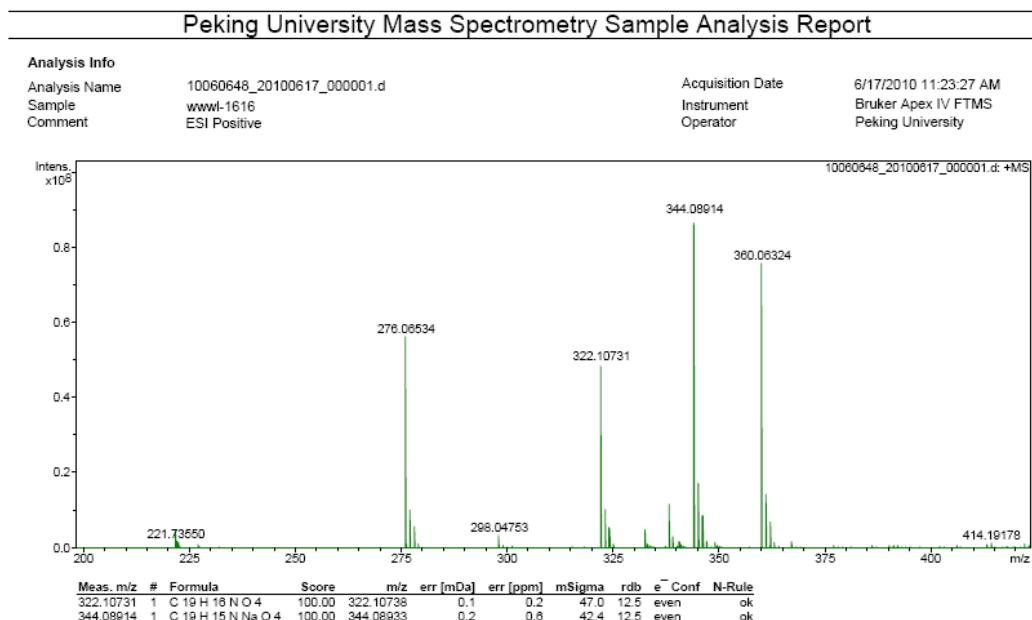
The HRMS spectra of **3a** for the reaction under  $^{18}\text{O}_2$  (97%).
