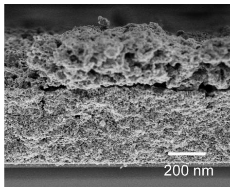
**Fig. S5** Cross-sectional SEM image of the working photoanode.
