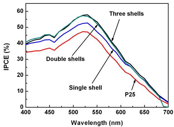
**Fig. S6** IPCE curves of the photoanode composing of P25/ the hierarchical  $\text{TiO}_2$  nanoplates with different shell numbers.
