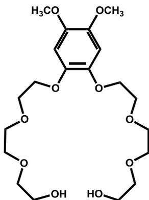
4,5-Dimethoxycatechol (6.00 g, 0.0353 mol), CsCO<sub>3</sub> (57.4 g, 0.1763 mol), and 2-[2-(2-chloroethoxy)ethoxy]ethanol (15.4 mL, 0.1059 mol) were dissolved in anhydrous MeCN (500
