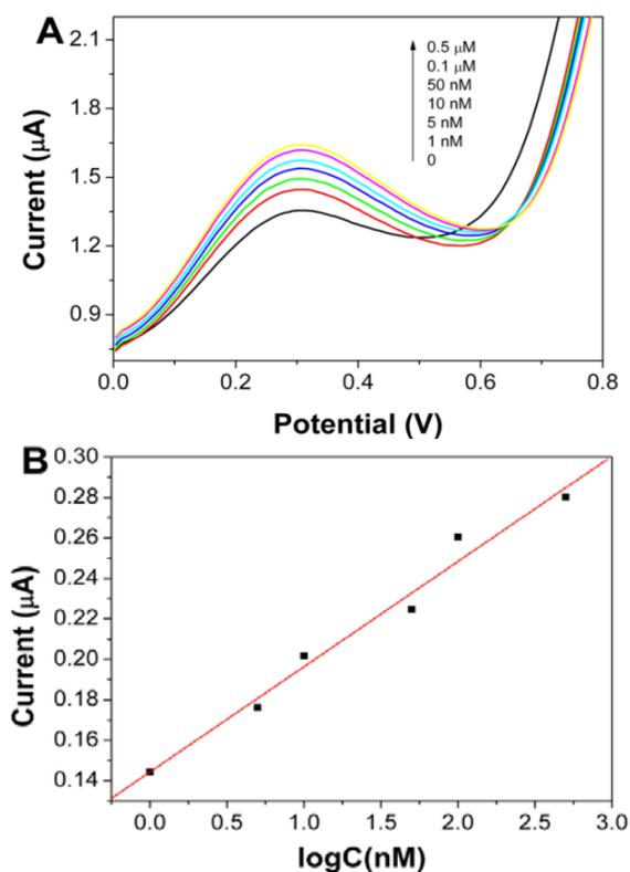
**Fig. S1** A) Typical SWVs of DNAzymes/gold electrode to different *L*-histidine concentration from 1 nM to 0.5  $\mu\text{M}$ . b) Linear relationship between the peak currents and *L*-histidine concentration.
