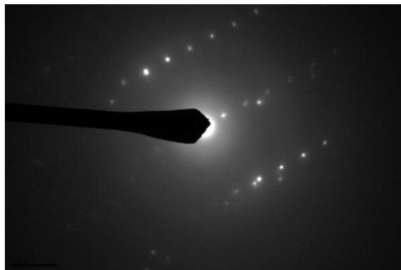
Figure S1. Selected area electron diffraction pattern for quartz nanosphere.
