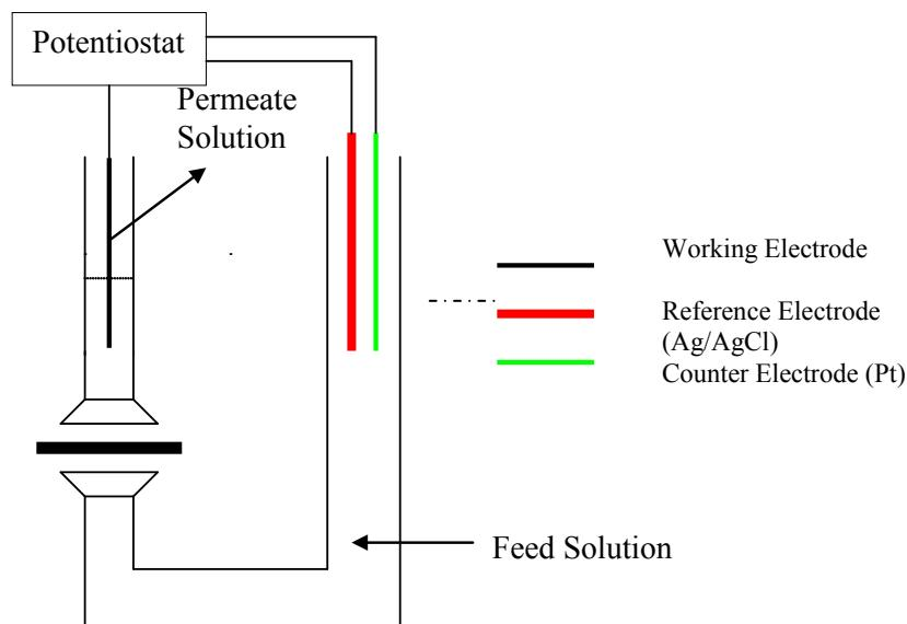
Figure S2.1 Experimental set-up for studying electro-phoretic and electro-osmotic transport across carbon nanotube membranes. The permeate concentration is measured as a function of time by UV-vis spectroscopy. The experiments are carried out potentiostatically using a Potentiostat/Galvanostat (Model 263A, Princeton Applied Research). Both the working and counter electrode are Pt wires and the reference electrode is an Ag/AgCl (sat. KCl) electrode.
