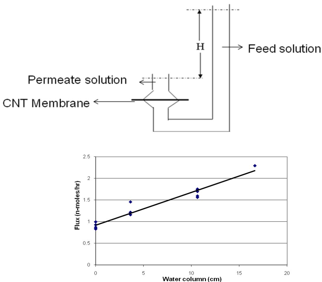
Figure S1. Schematic of the experimental set-up to study pressure driven water transport using a UV-active probe molecule  $\text{Ru}(\text{bipy})_3^{2+}$  as the feed solution. The extra height of the feed solution (H), provides the requisite pressure for measuring the convective transport properties of carbon nanotube membranes. Below: Plot of experimental data of pressure driven transport in CNT membranes.
