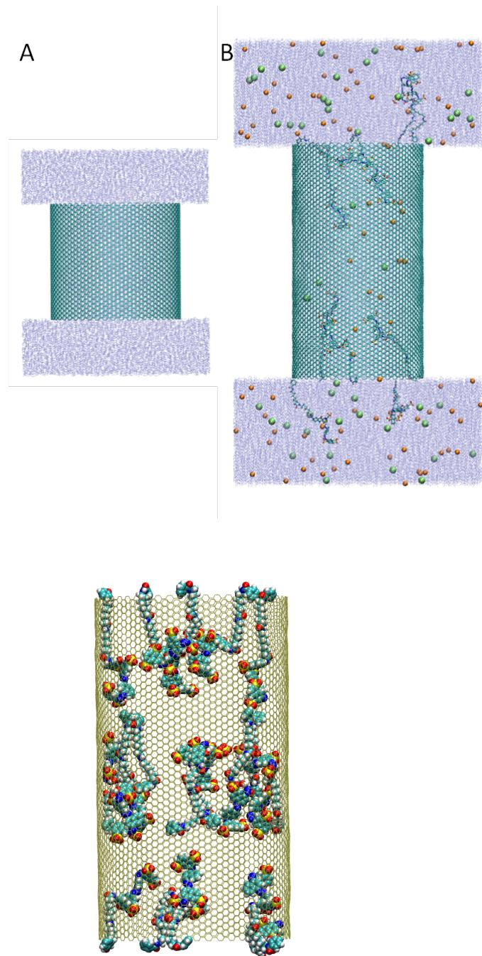
Figure S3 A snapshot of the simulation systems used to study fluid flow in (A) smooth polar CNTs, (B) tip functionalised and (C) core functionalised CNTs. Water is not shown in C so as not to obscure the locations of the functional groups attached to the CNT.
