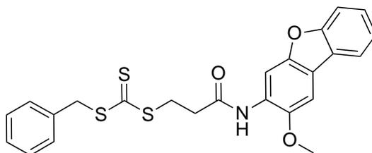
Chain transfer agent **CTA1** was synthesised by an amidation reaction between 3-benzylsulfanylthiocarbonylsulfanyl propionic acid and 3-amino-2-methoxy dibenzofuran (see Scheme 1).<sup>[3]</sup> A 50 mL RB flask was charged with 3-benzylsulfanylthiocarbonylsulfanyl propionic acid (0.54 g, 2 mmol), *N,N'*-dicyclohexylcarbodiimide (1.03 g, 5 mmol), 3-amino-2-methoxydibenzofuran (0.36 g, 1.67 mmol) and dry dichloromethane (25 mL). The reaction mixture
