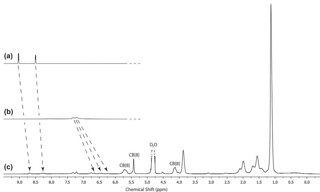
Figure S2: Partial <sup>1</sup>H NMR spectra (500 MHz, D<sub>2</sub>O) at 20 °C of **M<sub>2</sub>V** (a) and **P1** (b), and full <sup>1</sup>H NMR spectrum (500 MHz, D<sub>2</sub>O) at 20 °C of **P1+M<sub>2</sub>V**⊂**CB[8]** (c). The signals corresponding to the resonance of the solvent protons have been truncated for clarity.
