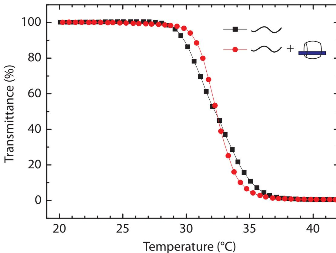
Figure S4: Thermosensitive phase transition plots of **P2** (0.2 mM in water) in the absence (black squares) and presence (red circles) of  $M_2V\subset CB[8]$ . Recorded at 600 nm and at a heating rate of 1 °C/min.
