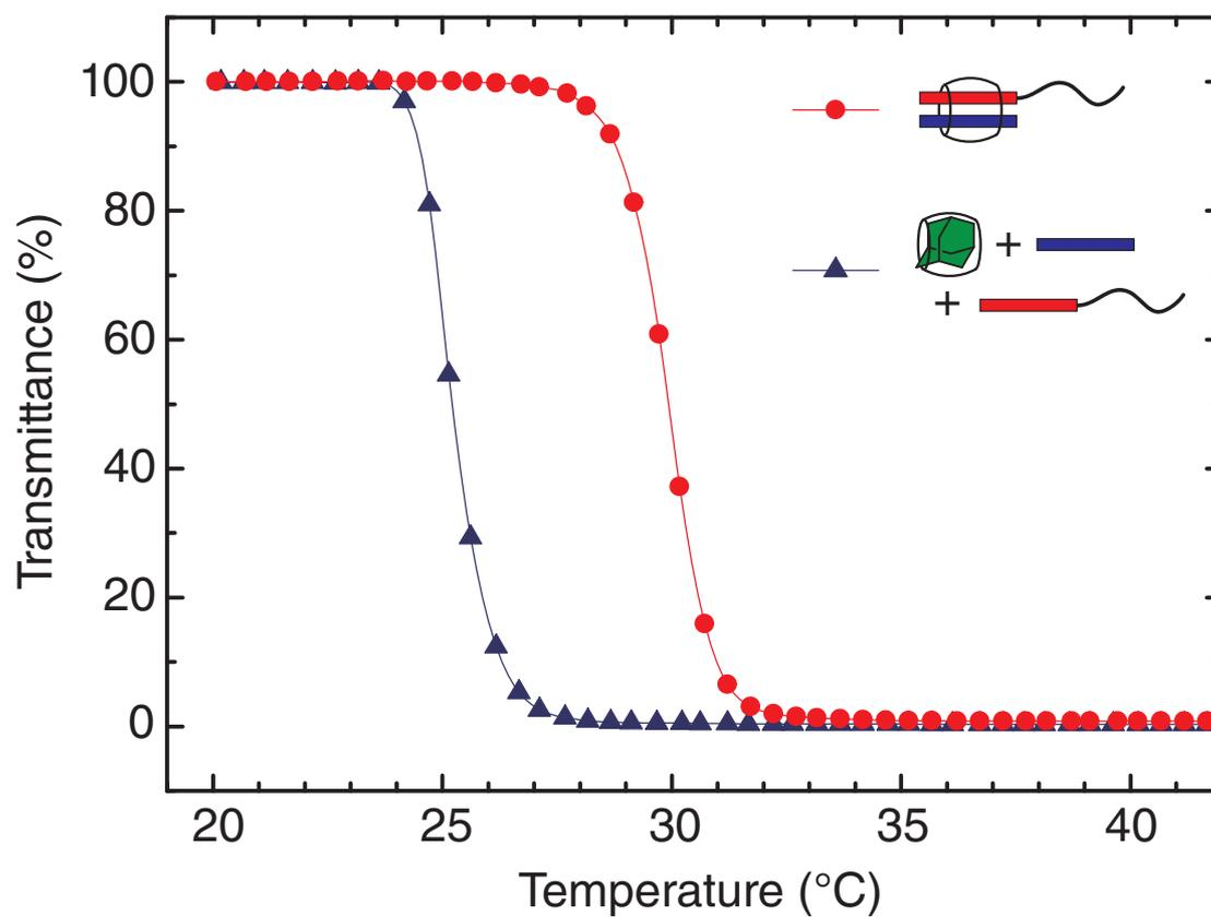
Figure S6: Thermosensitive phase transition plot of **P1+M<sub>2</sub>V⊂CB[8]** (0.2 mM in water) in the absence (red circles) and presence (blue triangles) of 1-aminoadamantane. Recorded at 600 nm and at a heating rate of 1 °C/min.
