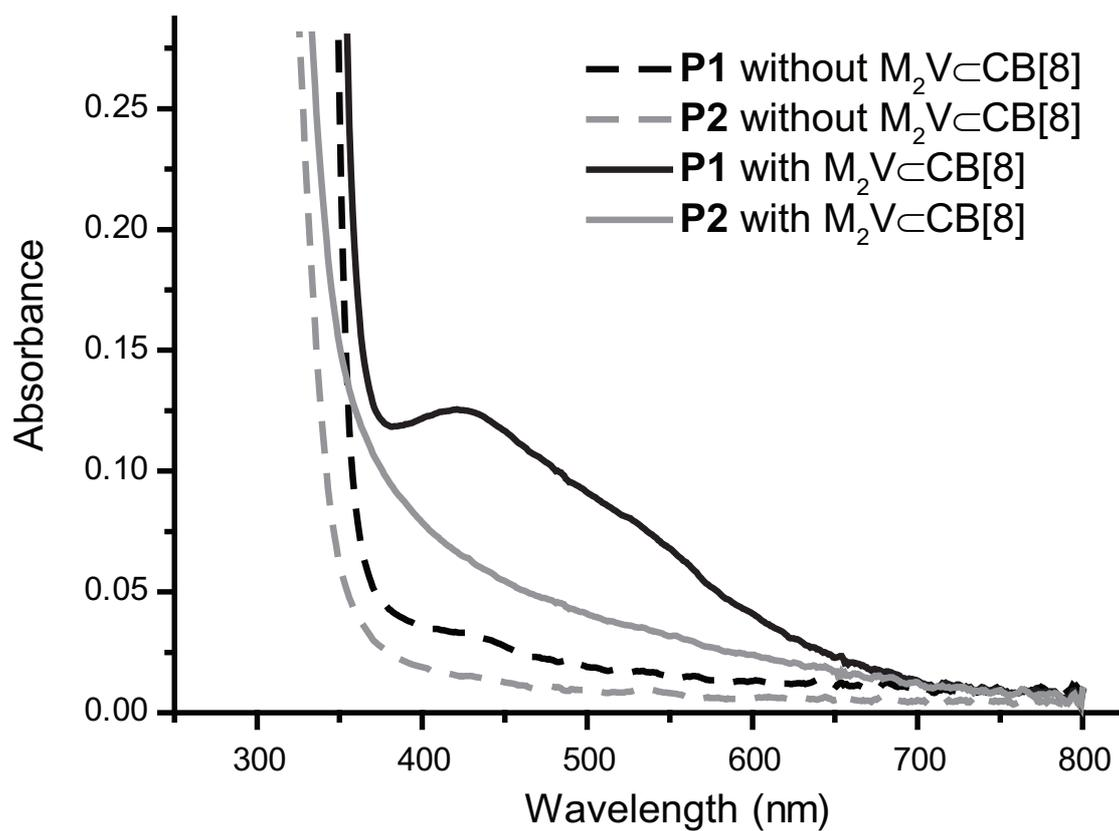
Figure S3: UV/vis spectra of aqueous solutions of **P1** (dotted black line), **P2** (dotted grey line), **P1** in the presence of 1 equiv of **M<sub>2</sub>V⊂CB[8]** (solid black line) and **P2** in the presence of 1 equiv of **M<sub>2</sub>V⊂CB[8]** (solid grey line).
