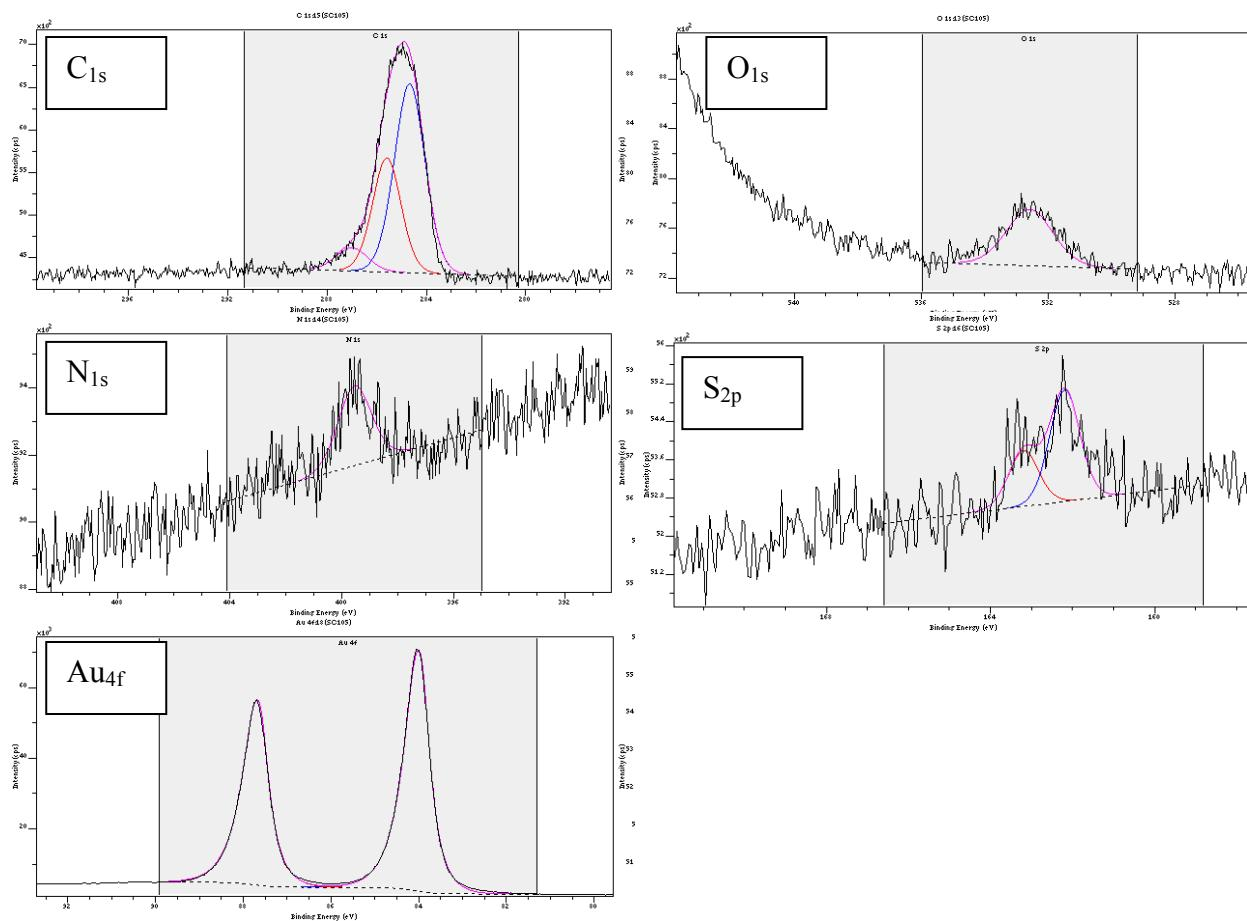
Figure S5. XPS spectra of C<sub>1s</sub>, O<sub>1s</sub>, N<sub>1s</sub>, Au<sub>4f</sub> and S<sub>2p</sub>
