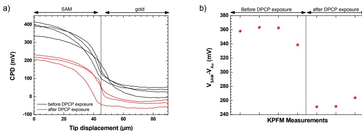
Fig. S7. (a) CPD measured along a line as shown in Fig. S6 for the Au functionalized with **3** before (black curves) and after (red curves) reaction with DPCP. **3** to 4 measurements were done at different places for each sample. (b) Potential difference calculated between  $V_{SAM}$  at  $x=0$  on Fig. S7a and  $V_{Au}$  at  $x = 90$   $\mu\text{m}$ .
