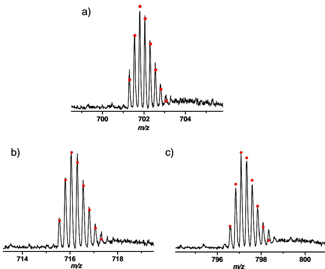
**Figure S2.** Isotopic models (dots, for which the values of  $x$  and  $y$  correspond to the  $m/z$  value and intensity of the respective isotopic ion peak, respectively) and mass spectra (lines) for platinumated peptide a) T3-**1''**:
