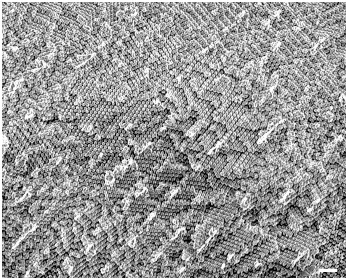
Figure S4. SEM of a cracked wing scale with the cubic structure visible. As seen here the replication of the internal structure occurs on a large scale. Not also the filling factor being higher than that of the butterfly (Fig. 2). Scale bar is 1 \mu\text{m} .
