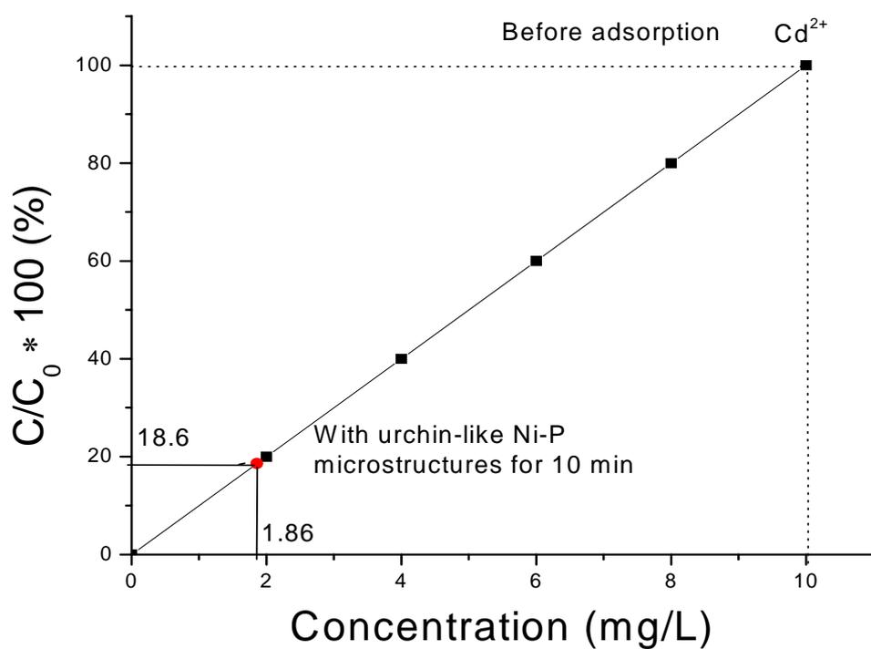
Figure S7. The concentration of the solution containing  $Pb^{2+}$  or  $Cd^{2+}$ : (—■—) calibration curve and (.....) before and (—) after adsorption with urchin-like Ni-P microstructures for 10 min.
