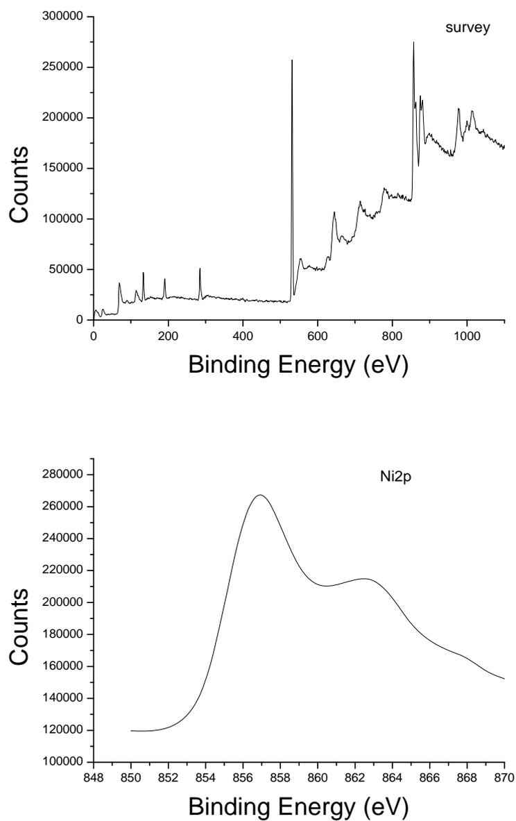
Figure S2 Survey X-ray photoelectron spectra of urchin-like Ni-P microstructures and high resolution XPS of Ni.
