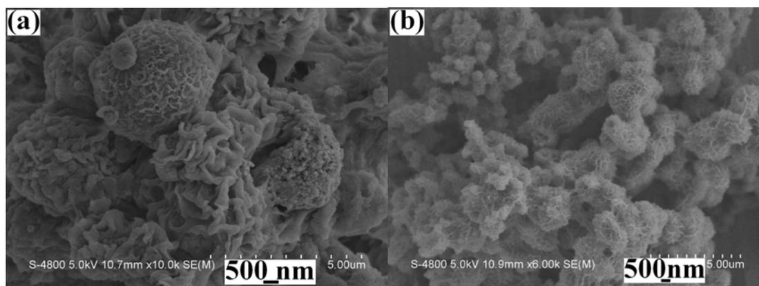
Figure S4. FE-SEM images of Ni-P microstructures prepared from the systems containing various water/DMF volume ratios at 160°C for 16 h: (a) 13.5:6.5 and (b) 6.5:13.5.
