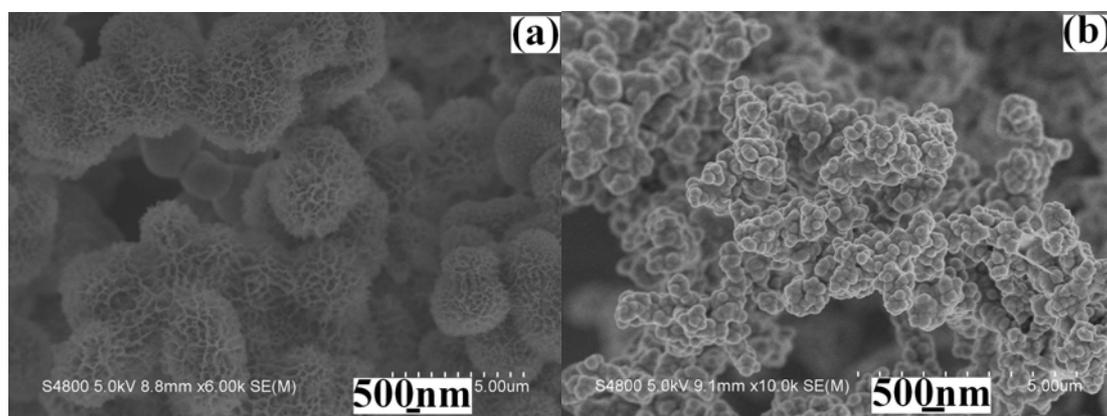
Figure S5. FE-SEM images of Ni-P microstructures prepared under the same system at different temperatures for 16 h: (a) 140°C and (b) 180°C.
