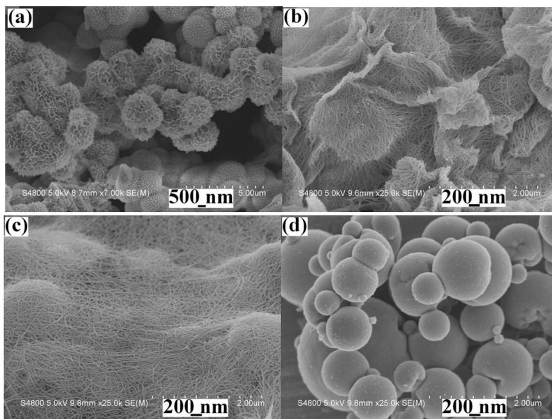
Figure S3. FE-SEM images of Ni-P microstructures prepared from the systems containing various  $\text{Ni}^{2+}/\text{H}_2\text{PO}_2^-$  molar ratios at 160°C for 16 h: (a) 4:1, (b) 1:1, (c) 2:3 and (d) 1:5.
