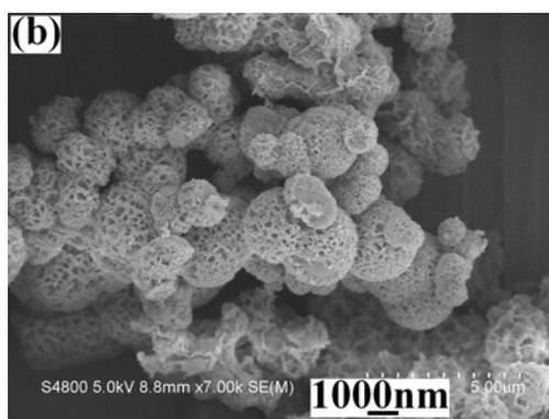
**Figure S1.** (a) XRD patterns of the products: the below curve is the pattern of the product prepared at 160 °C for 16 h and the upper curve is the one of the product treated at 500 °C for 2 h. (b) A representative SEM image of the product treated at 500 °C for 2 h.
