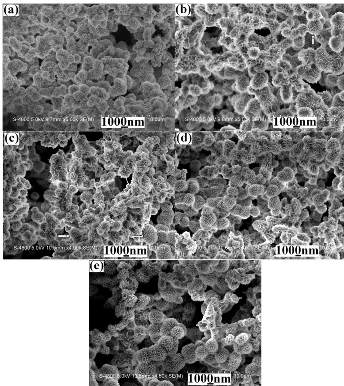
Figure S6. FE-SEM images of Ni-P microstructures prepared under the same system at 160°C for different durations: (a) 30 min, (b) 4 h, (c) 7 h, (d) 10 h and (e) 13h.
