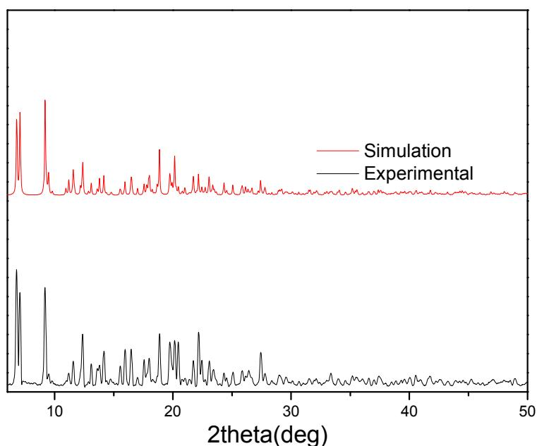
**Fig. S5** X-ray powder diffraction patterns for **1b**: red, calculated from single-crystal X-ray data; black, experimental data.
