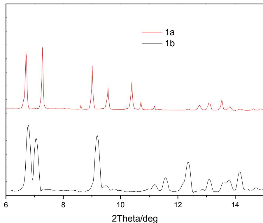
**Fig. S6** A comparison of X-ray powder diffraction patterns for **1a** and **1b** at low angle.
