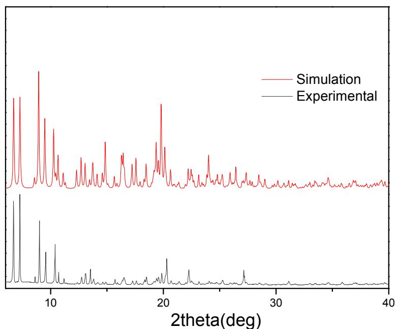
**Fig. S4** X-ray powder diffraction patterns for **1a**: red, calculated from single-crystal X-ray data; black, experimental data.
