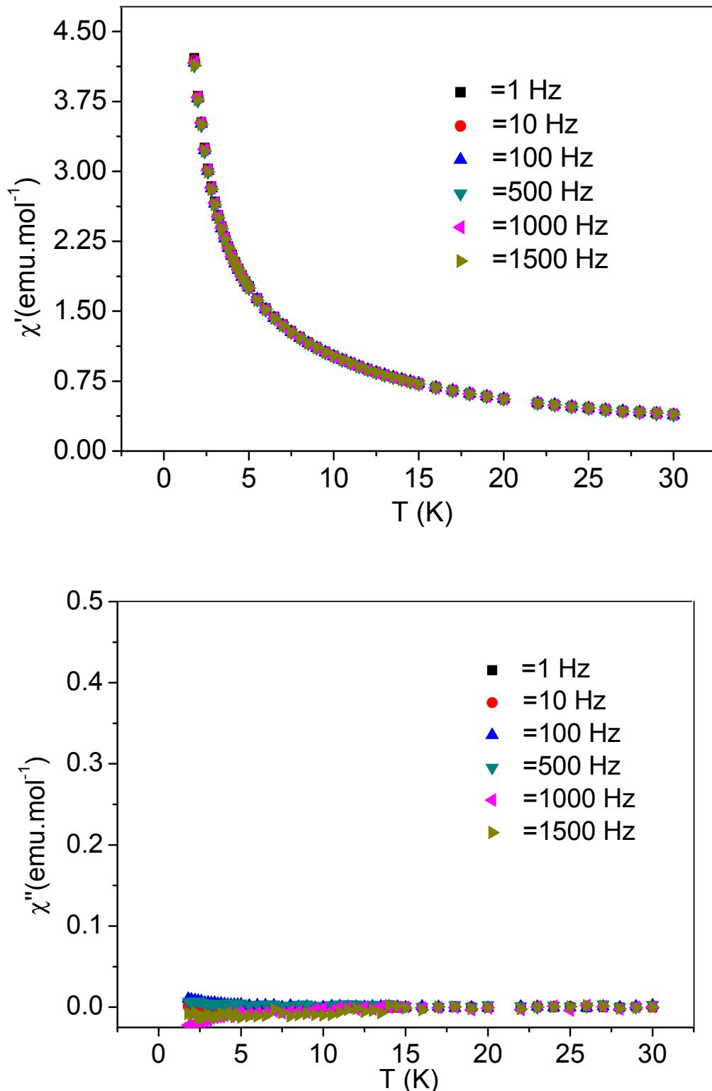
**Fig. S11** In-phase (top,  $\chi_m'$ ) and out-of-phase (bottom,  $\chi_m''$ ) dynamic magnetic susceptibilities of **1b** measured in a 3 Oe AC magnetic field with a 2000 Oe dc-field.
