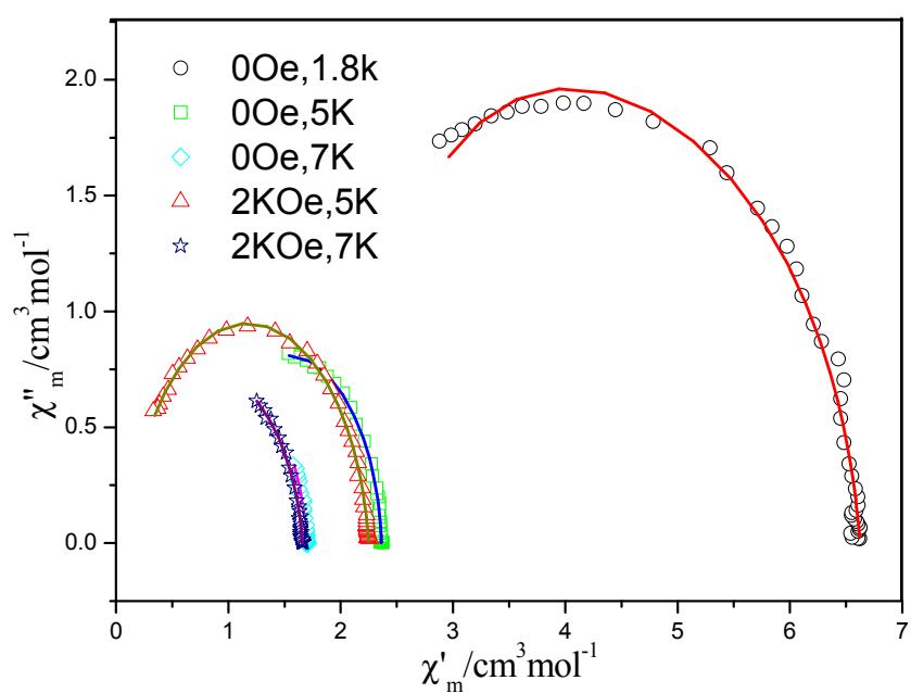
**Fig. S10** Cole-Cole plots for ac susceptibility collected under  $H_{dc} = 0$  Oe and 2 kOe for **1a**. The solid lines represent the fitting with a Debye mode. In the plots,  $\alpha = 0.12$ , 0.04, 0.06 at 1.8, 5 and 7 K with  $H_{dc} = 0$  Oe;  $\alpha = 0.08$ , 0.07 at 5 and 7 K with  $H_{dc} = 2$  kOe.
