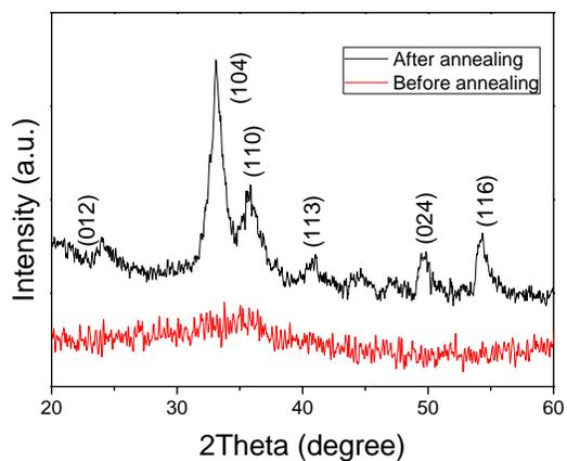
Fig. S1. XRD patterns of the samples before and after annealing in air.
