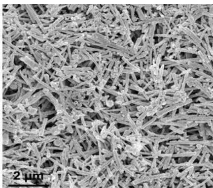
Fig. S2. Overview FESEM image of Fe(OH)<sub>x</sub> nanotubes.
