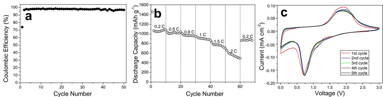
Fig. S4. (a) Coulombic efficiency of  $\alpha$ -Fe<sub>2</sub>O<sub>3</sub> nanotubes cycled between 0.01 – 3V at a 0.5C rate. (b) Rate capability of  $\alpha$ -Fe<sub>2</sub>O<sub>3</sub> nanotubes between 0.01 – 3.0 V; (c) cyclic voltammograms at a scan rate of 0.5 mV s<sup>-1</sup> between 0.01 – 3.0 V. All potentials are with reference to Li/Li<sup>+</sup>.
