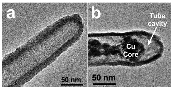
Fig. S3. TEM image showing (a) capped end of Fe(OH)<sub>x</sub> nanotubes; (b) one end of a nanotube with residual Cu, suggesting the formation of inner cavities before complete dissolution of the Cu template.
