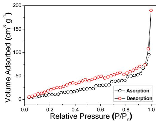
Fig. S5. N<sub>2</sub> adsorption/desorption isotherm of  $\alpha$ -Fe<sub>2</sub>O<sub>3</sub> nanotubes.
