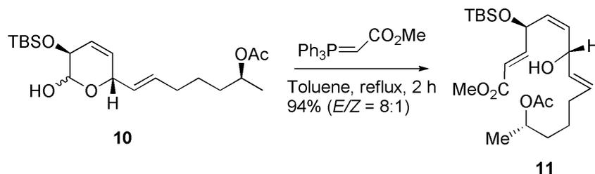
To a stirred solution of **10** (9.7 mg, 25.2  $\mu\text{mol}$ ) in toluene (0.3 mL) was added methyl (triphenylphosphoranylidene) acetate (42.2 mg, 0.126 mmol) at room temperature, and then the mixture was heated to reflux. After being stirred for 2 h, the resultant mixture was concentrated in vacuo. The residue was purified by silica gel column chromatography (hexane / AcOEt = 90 / 10) to afford the **Z-isomer** (1.2 mg, 10%) as a colorless oil and **11** (9.2 mg, 84%) as a colorless oil;
