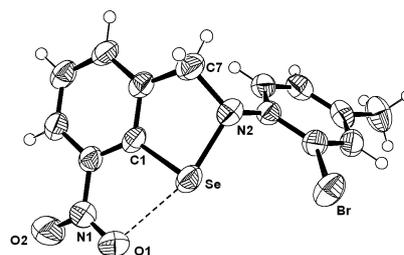
Figure 7. Molecular structure of **30**. Thermal ellipsoids are set at 50 % probability. Significant bond lengths [Å] and angles [°]: Se···O1 2.686(3); Se—N2 1.905(3); Se—C1 1.880(3); O1···Se—N2 155.61(10); C1—Se—N2 88.11(12); C7—N2—Se 107.00(19).
