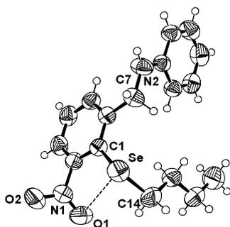
Figure 4. Molecular structure of **21**. Thermal ellipsoids are set at 50 % probability. Significant bond lengths [Å] and angles [°]: Se···O1 3.295(9); Se—C1 1.924(2); Se—C14 1.978(3); O1···Se—C7 115.93(6); C1—Se—C14 100.00(11).
