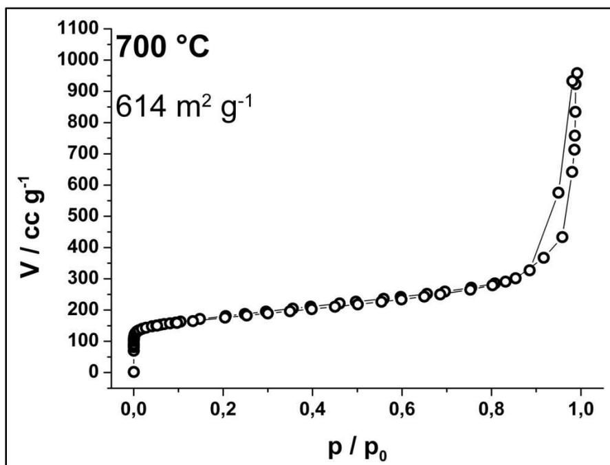
Fig. S 6: Nitrogen sorption isotherm of S-doped carbonaceous material synthesised at 700 °C.
