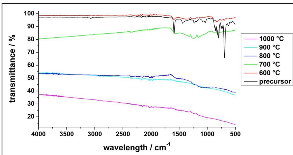
Fig. S 1: FT-IR spectra of the thienyl-based precursor and the samples thermally treated at varying temperatures.
