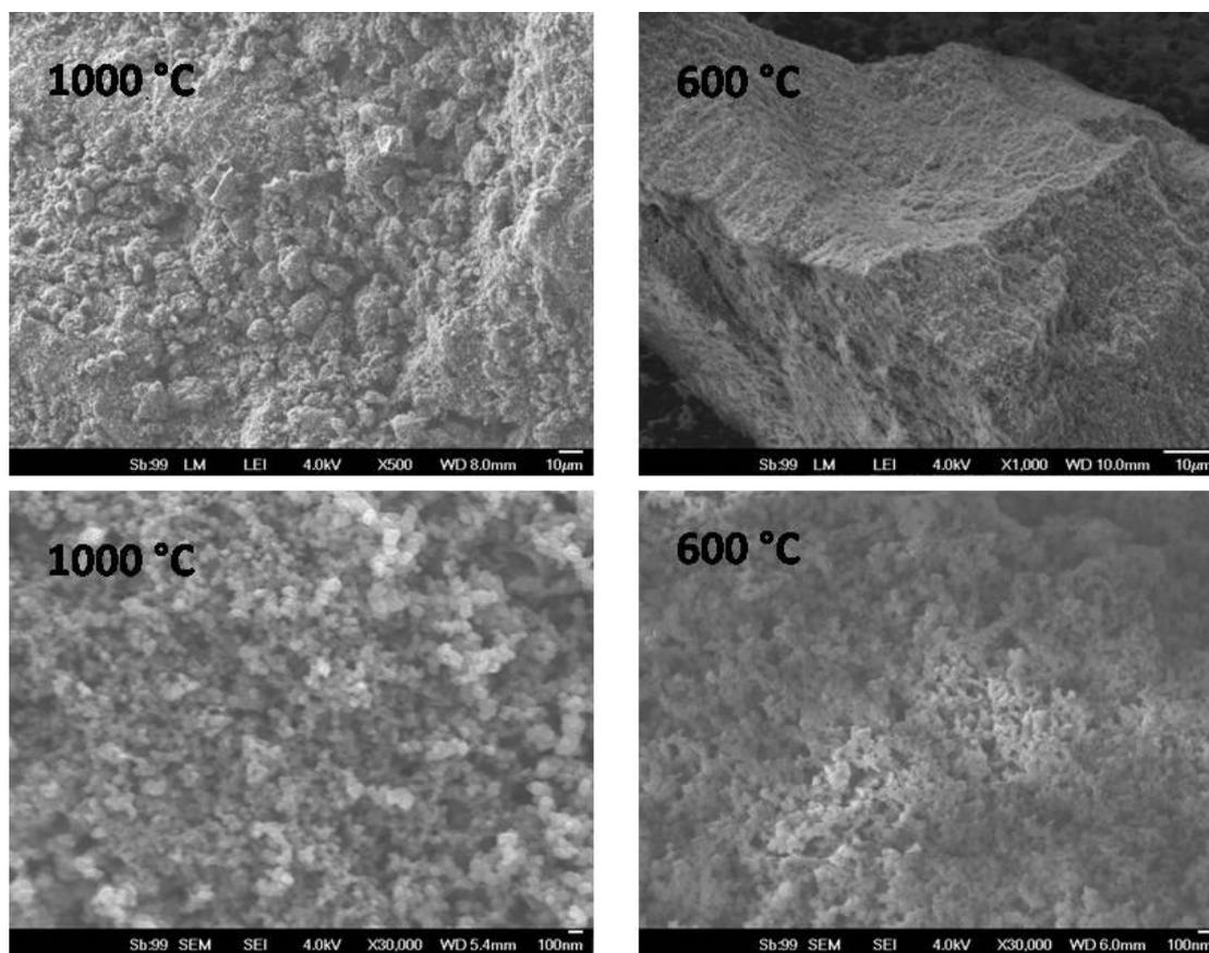
Fig. S 3: SEM micrographs of S-doped carbonaceous materials synthesized at 600 °C and 1000 °C.
