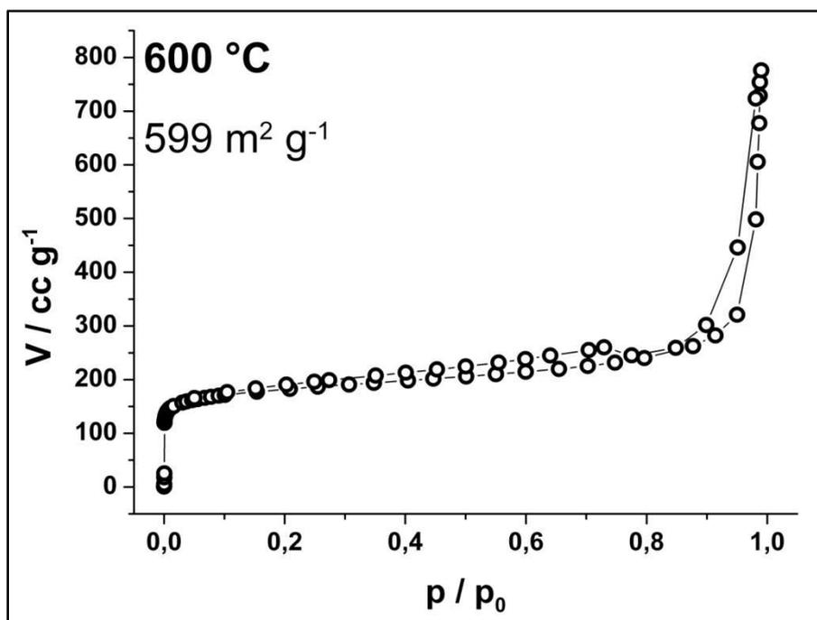
Fig. S 5: Nitrogen sorption isotherm of S-doped carbonaceous material synthesised at 600 °C.
