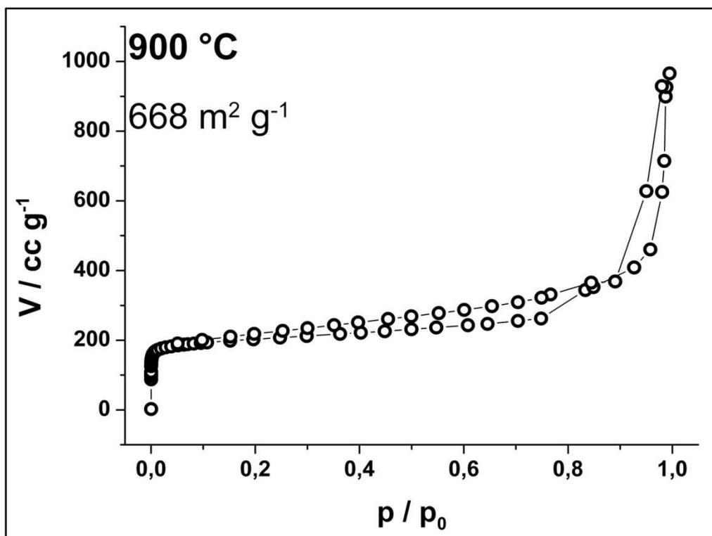
Fig. S 8: Nitrogen sorption isotherm of S-doped carbonaceous material synthesised at 900 °C.
