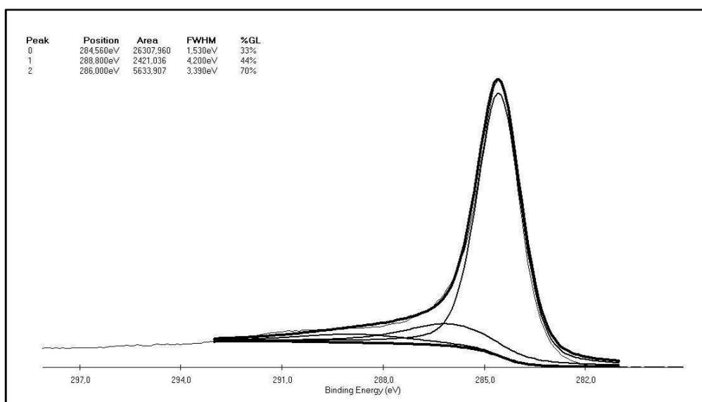
Fig. S 2: Deconvoluted XPS-spectrum of the C-1s orbital, measured on the material synthesised at 1000 °C.
