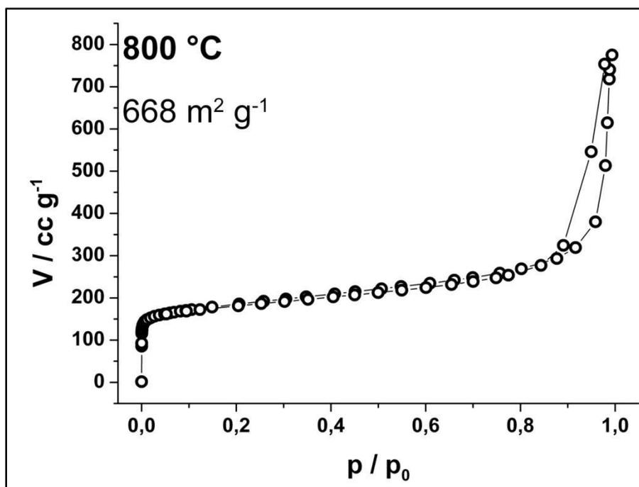
Fig. S 7: Nitrogen sorption isotherm of S-doped carbonaceous material synthesised at 800 °C.
