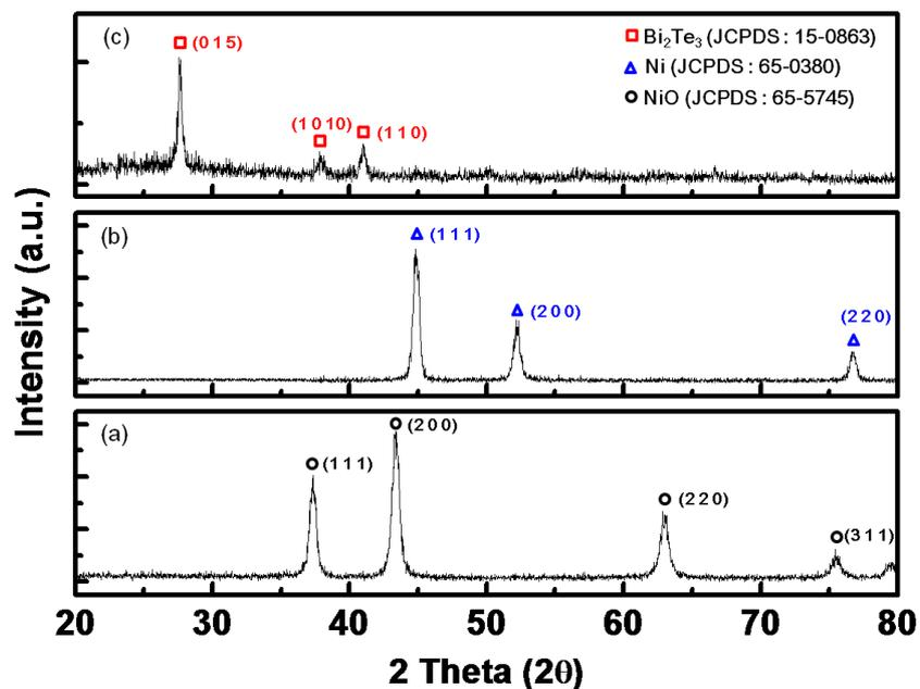
**Figure S.1** XRD patterns of synthesized nanofibers: (a) NiO nanofibers synthesized by calcinating PVP/Ni acetate nanofibers at 500°C in air, (b) Ni nanofibers after thermal reduction of NiO nanofibers at 400°C in 5% H<sub>2</sub>/N<sub>2</sub> and (c) Bi<sub>2</sub>Te<sub>3</sub> nanotubes fibers after galvanic displacement reactions.
