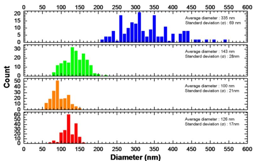
**Figure S.4** Diameter distribution of the synthesized nanofibers: (a) PVP/Ni acetate, (b) NiO, (c) Ni, and (d) Bi<sub>2</sub>Te<sub>3</sub> nanofibers.
