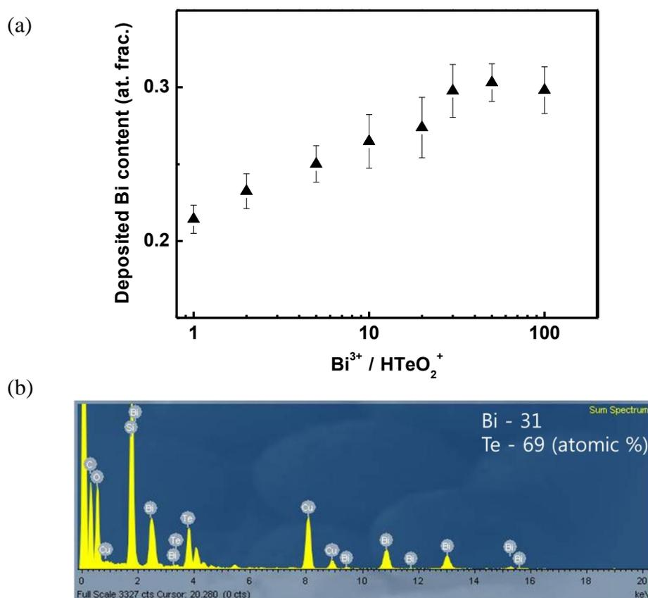
**Figure S.3.** (a) Dependence of the deposited Bi content of  $\text{Bi}_x\text{Te}_y$  nanofibers as a function of  $[\text{Bi}^{3+}]/[\text{HTeO}_2^+]$  ratio.  $[\text{Bi}^{3+}]$  was varied from 1 mM to 100 mM while fixing the  $[\text{HTeO}_2^+]$  and  $[\text{HNO}_3]$  at 1 mM and 1 M, respectively at room temperature. (b) Typical EDS spectra of synthesized  $\text{Bi}_x\text{Te}_{1-x}$  nanofibers.
