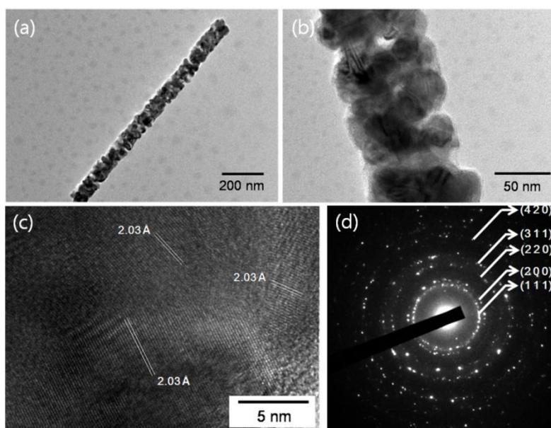
**Figure S.2.** HR-TEM images (a, b, c) and corresponding SAED pattern (d) of the nickel nanofibers.
