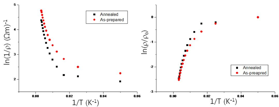
**Fig. S.6.** TCR analysis of  $Bi_xTe_y$  nanotubes before and after the annealing process in a reducing environment (5%  $H_2$  + 95 %  $N_2$ ) at 473 K for 2 hours.
