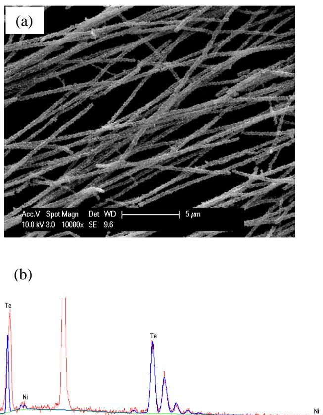
**Figure S.5** SEM image of (a) hollow Te nanofibers synthesized by galvanic displacement of Ni nanofibers with corresponding (b) EDS spectra.
