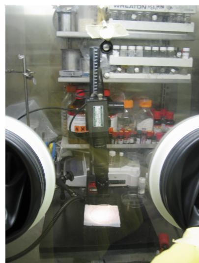
**Figure S2.** Photograph showing the set-up used to mount the crystals of **3** into a capillary tube. A microscope is needed inside the dry-box as part of the contamination control and safety procedures required when handling the  $^{239}\text{Pu}$  radioisotope.
