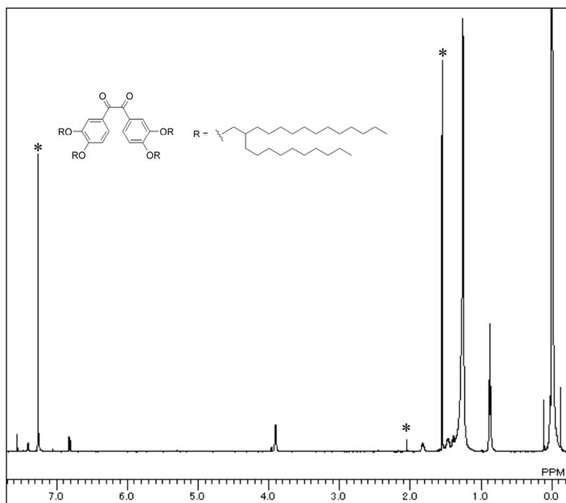
Fig.S2  $^1\text{H}$ -NMR spectrum of 3,3',4,4'-tetra-2-decyl-tetradecyloxybenzil in  $\text{CDCl}_3$  (\* solvent peaks).
