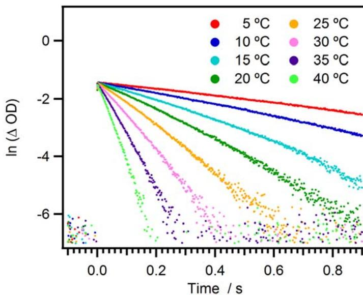
Fig. S14 First-order kinetic profiles of the colored species **1R** monitored at 400 nm in degassed benzene (**1**:  $2.1 \times 10^{-4}$  M, light path length: 10 mm). The measurements were performed in the temperature range from 5 °C to 40 °C.
