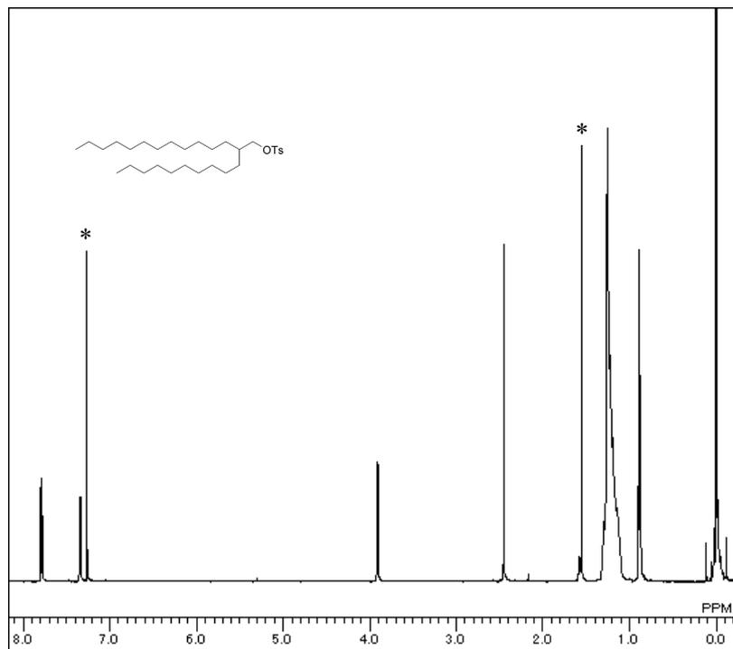
Fig. S1  $^1\text{H}$ -NMR spectrum of 2-decyl-tetradecyloxy tosylate in  $\text{CDCl}_3$  (\* solvent peak).
