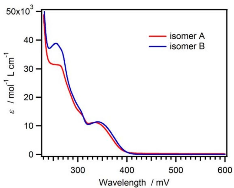
Fig. S12 UV-vis absorption spectra for **1** in acetonitrile; (red) isomer A, (blue) isomer B.
