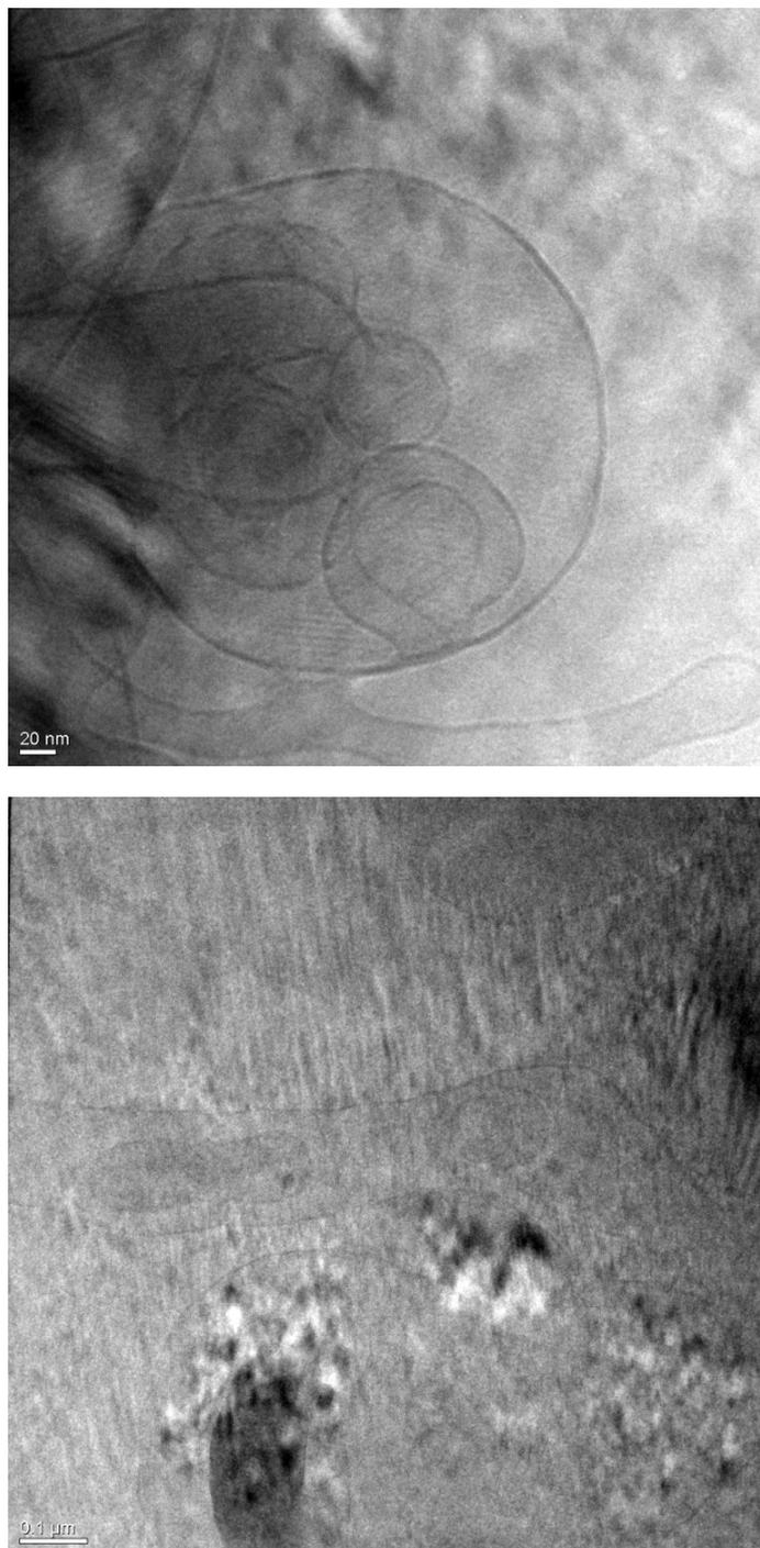
Fig. S21 Cryo-TEM images of the oligo-lamellar vesicles in water.
