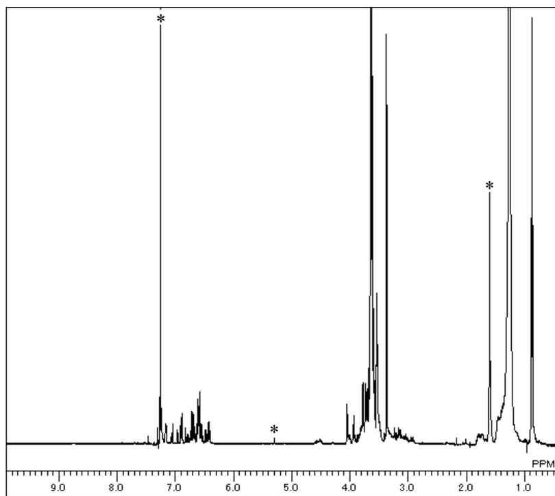
Fig. S7  $^1\text{H}$ -NMR spectrum of compound **1** (isomer B) in  $\text{CDCl}_3$  (\* solvent peak).
