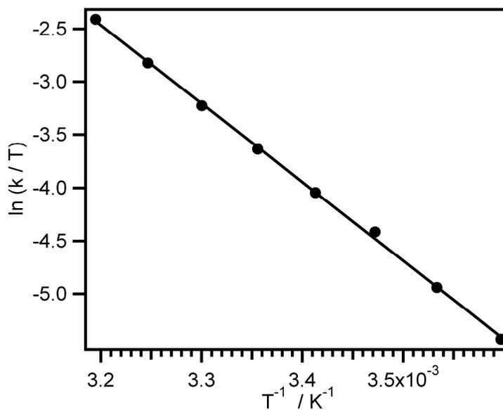
Fig. S15 Eyring plot for the thermal back-reaction of the colored species **1R**.
