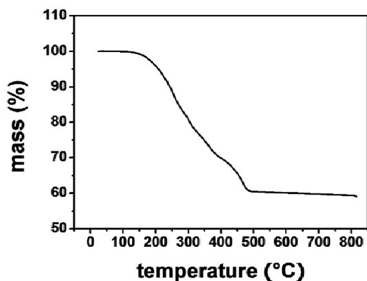
**Fig. S4** TGA diagram of dried NaYF<sub>4</sub>:20%Yb<sup>3+</sup>, 2%Tm<sup>3+</sup> nanoparticles.
