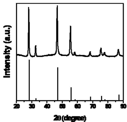
**Fig. S1** (top) powder XRD spectrum of synthesized colloidal NaYF<sub>4</sub>:Yb<sup>3+</sup>,Tm<sup>3+</sup> NP. (bottom) reference powder XRD spectrum of α-NaYF<sub>4</sub> face-centered cubic crystal (JCPDS no. 77-2042).
