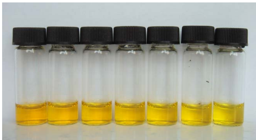
Fig.S12 Photograph showing the photocatalytic degradation under visible light for 0 min, 20 min, 40 min, 60 min, 80 min, 100 min and 120 min (from left to right respectively).
