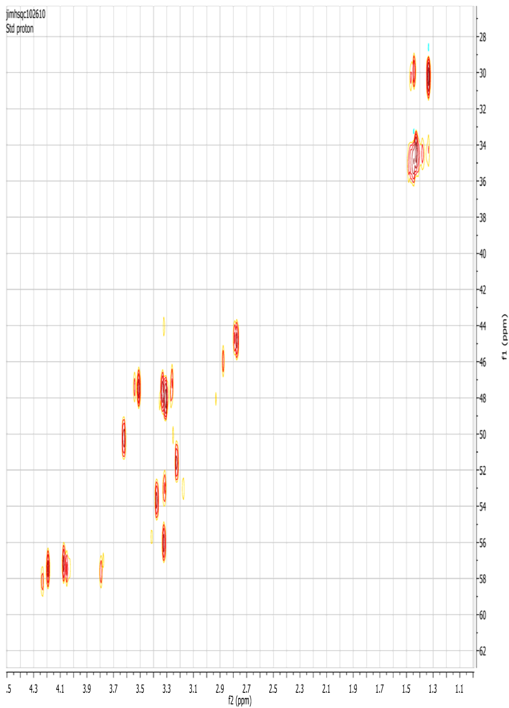
Fig. S8 HSQC (Heteronuclear Single Quantum Coherence) spectrum of 4 (benzene- d_6 , 26 °C). It gives the correlation between ^1\text{H} and ^{13}\text{C} atoms that are bound to each other. f1 and f2 are ^{13}\text{C} and ^1\text{H} NMR axes, respectively.
