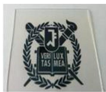
**Figure S4.** Photographs of graphene thin film on glass
