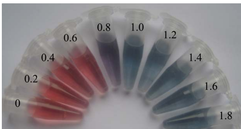
Fig. S5 Visual colorimetric change of the MPA-stabilized Au NPs upon addition of streptomycin with different concentrations (0, 0.2, 0.4, 0.6, 0.8, 1.0, 1.2, 1.4, 1.6, and 1.8 \mu\text{M} ).
