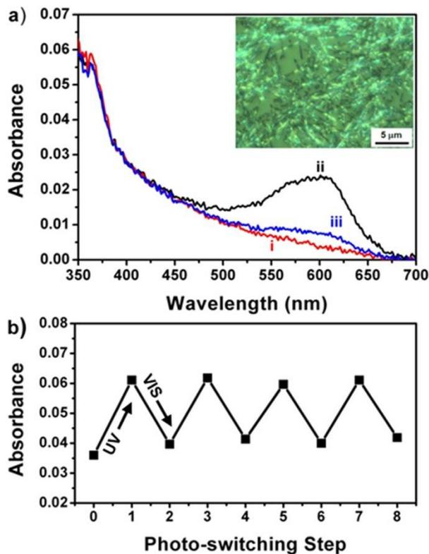
Fig. S1(a) UV-visible absorption spectra of a SO-PMMA nanowire mat following visible (i)-UV(ii)-visible (iii). Inset: optical image of cycled mat; (b) reversible modulation of mat absorption intensity following alternating steps of UV and visible irradiation.
