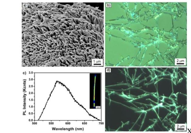
Fig. S2 (a) Scanning electron microscopy (SEM) image of freestanding SO-PMMA nanowire array; bright-field (b) and fluorescence (c) optical microscopy images PFA nanowire mat; (d) emission spectrum of individual PFA nanowire. Inset: fluorescence intensity image of PFA nanowire.
