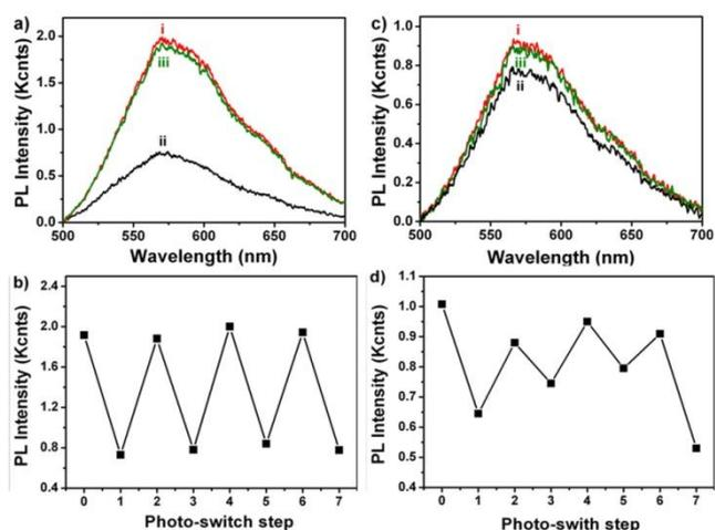
**Fig. SI3** Emission spectra from a single SO-PFA nanotube following vis (i)-UV (ii)-visible (iii) irradiation. (a) SO-PFA 20% w:w; (c) SO-PFA 1% w:w. Reversible modulation of nanotube emission following alternating steps of UV and visible irradiation. (b) SO-PFA 20% w:w; (d) SO-PFA 1% w:w.
