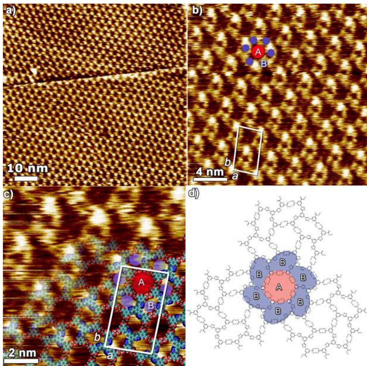
**Figure S3.** a) Large scale STM current image of **1** at the solid-liquid interface; b) small scale STM height image. c) Proposed CPK model of the **1**; (a, b, c) Tunneling parameters: Average tunneling current ( $I_t$ ) = 18pA, tip bias voltage ( $V_t$ ) = 600 mV, d) chemical representation of the proposed packing motif. In green Highlight of the 48 atoms perimeter central pore **A**, resulting from 6 di-hapto O-H...O H-bonding, and in blue the 42 atoms “smaller” pores **B**.
