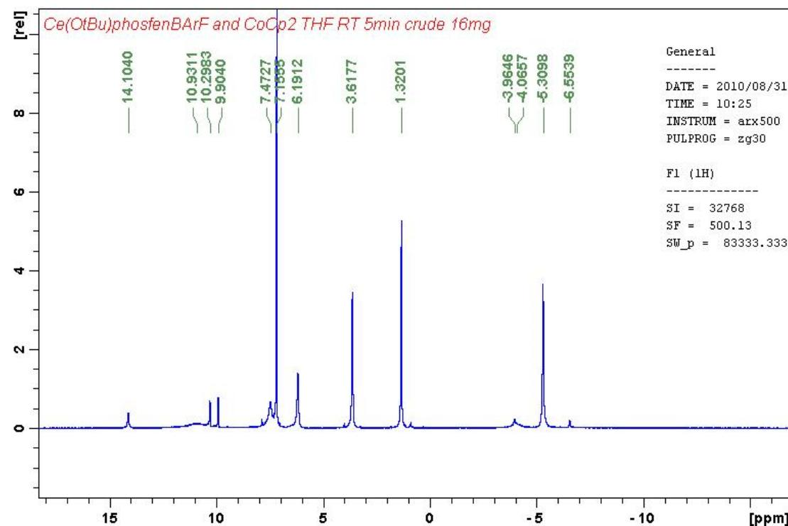
**<sup>1</sup>H NMR Spectrum for end-group analysis of poly(lactide) from 1-Ce(O<sup>t</sup>Bu) with 50 equivalents of L-lactide**
