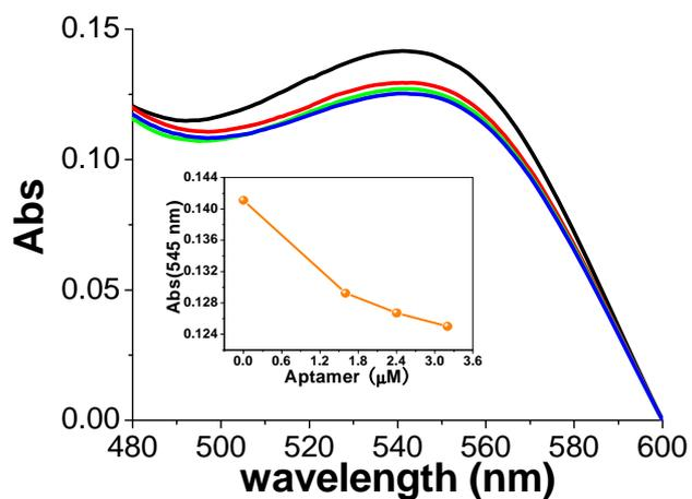
**Fig. S7.** UV/Vis spectra of MWNT-MC in the absence (black) or presence of 1.6  $\mu\text{M}$  (red), 2.4  $\mu\text{M}$  (green) and 3.2  $\mu\text{M}$  (blue) lysozyme aptamer. (Inset) Calibration curve corresponding to the absorbance value at 545 nm of MWNT-MC upon analyzing variable concentration of DNA aptamer.
