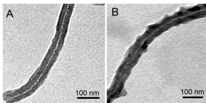
**Fig. S4.** High resolution transmission electron microscopy (HRTEM) images of (A) MWNT-COOH and (B) MWNT-MC.
