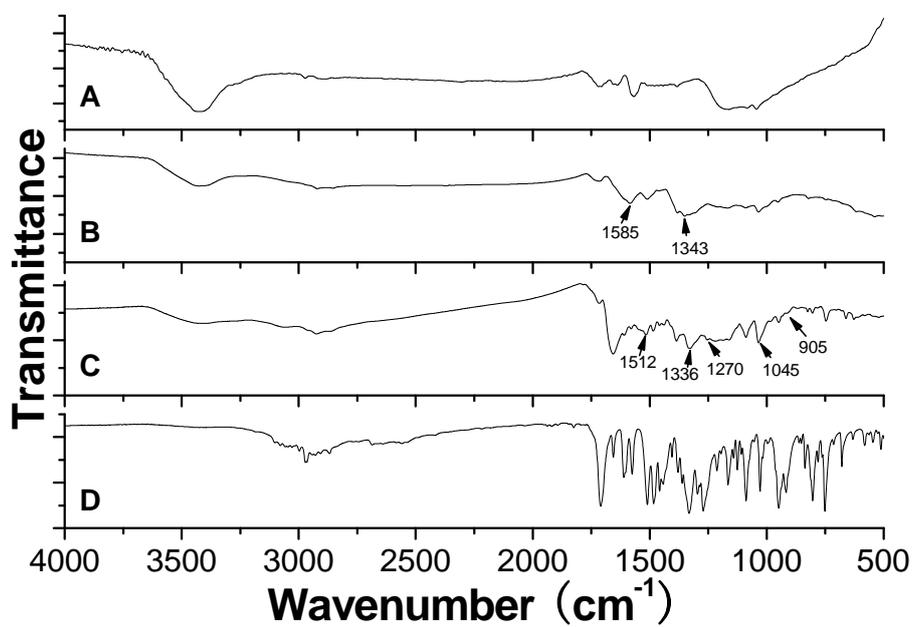
**Fig S2** FTIR of (A) MWNT-COOH, (B) MWNT-PAH, (C) MWNT-SP and (D) SP-COOH.
