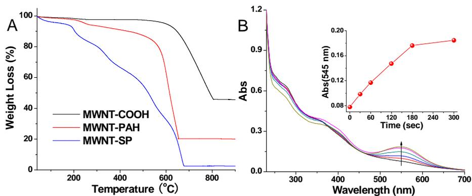
**Fig. S3** (A) Thermogravimetric analysis for MWNT-COOH (black), MWNT-PAH (red) and MWNT-SP (blue) in N<sub>2</sub> atmosphere with a ramp of 10 °C/min. (B) UV/Vis spectra of MWNT-SP irradiated by UV light for different time. (Inset) The absorption at 545 nm is depended on the time of irradiation.
