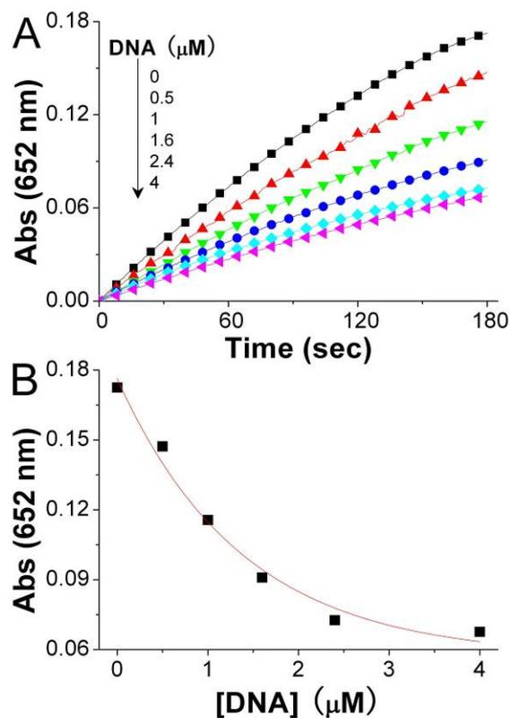
**Fig. S8** (A) Time-dependent absorbance changes of  $15 \mu\text{g}\cdot\text{ml}^{-1}$  MWNT-MC and  $10 \text{ ng}\cdot\text{ml}^{-1}$  HRP upon adding different concentration of DNA aptamer. (B) Calibration curve corresponding to the absorbance upon analyzing variable concentration of DNA aptamer after a fixed time interval of 3 min.
