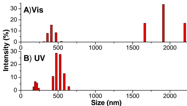
**Fig. S5** Size distribution determined by dynamic light scattering (DLS): (A) MWNT-SP and (B) MWNT-MC.
