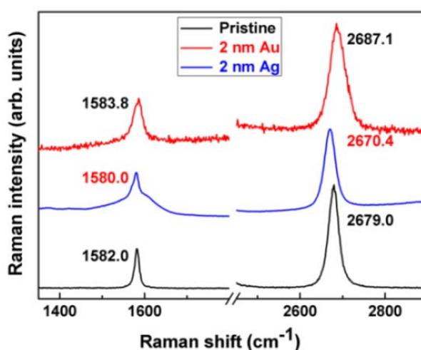
**Fig. S5.** The frequency shift of G peak in Raman spectra of 2 nm Au or Ag-decorated monolayer graphene.
