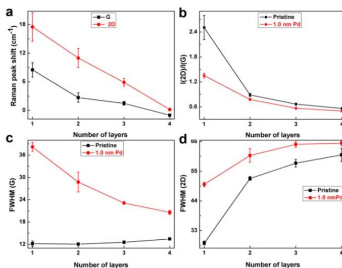
**Fig. S6.** The peak frequency shifts, intensity ratio ( $I_{2D}/I_G$ ) and full width at half maximums of G and 2D peaks in Raman spectra of 1.0 nm Pd-decorated n-layer
