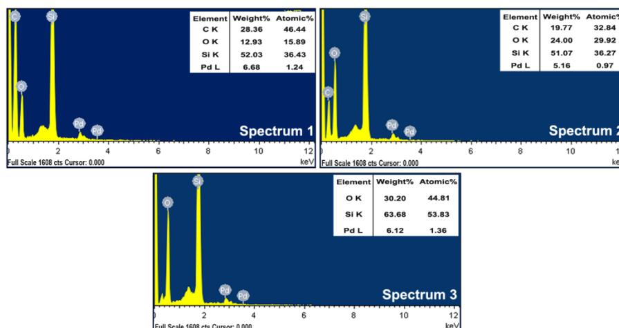
**Fig. S3.** EDX spectra showing the obvious Pd signals on thick, thin graphene, and substrate. Spectrum 1, 2 and 3 corresponds to EDX on the thick, thin graphene and the substrate, respectively.
