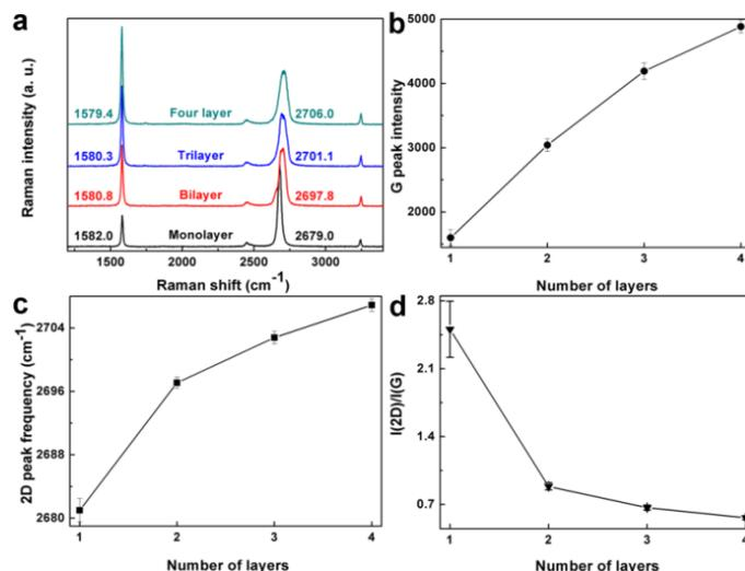
**Fig. S1.** The Raman spectra (a), G peak intensity (b), 2D peak frequency (c) and peak intensity ratio (d) of pristine n-layer graphenes (n = 1, 2, 3, 4), which are obviously dependent on the layer number of n-layer graphenes.
