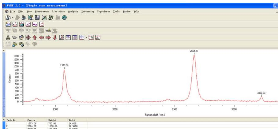
**Fig. 4** The parameters of Raman spectrum of Pd-decorated monolayer graphene given by the software of Raman spectroscopy.
