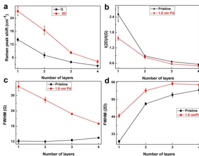
**Fig. S7.** The peak frequency shifts, intensity ratio ( $I_{2D}/I_G$ ) and full width at half maximums of G and 2D peaks in Raman spectra of 1.6 nm Pd-decorated n-layer graphenes compared with pristine graphenes.
