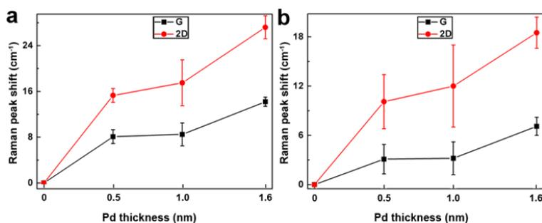
**Fig. S8.** The effects of Pd film thickness on charge transfer between graphenes and Pd. (a) Monolayer and (b) bilayer graphene.
