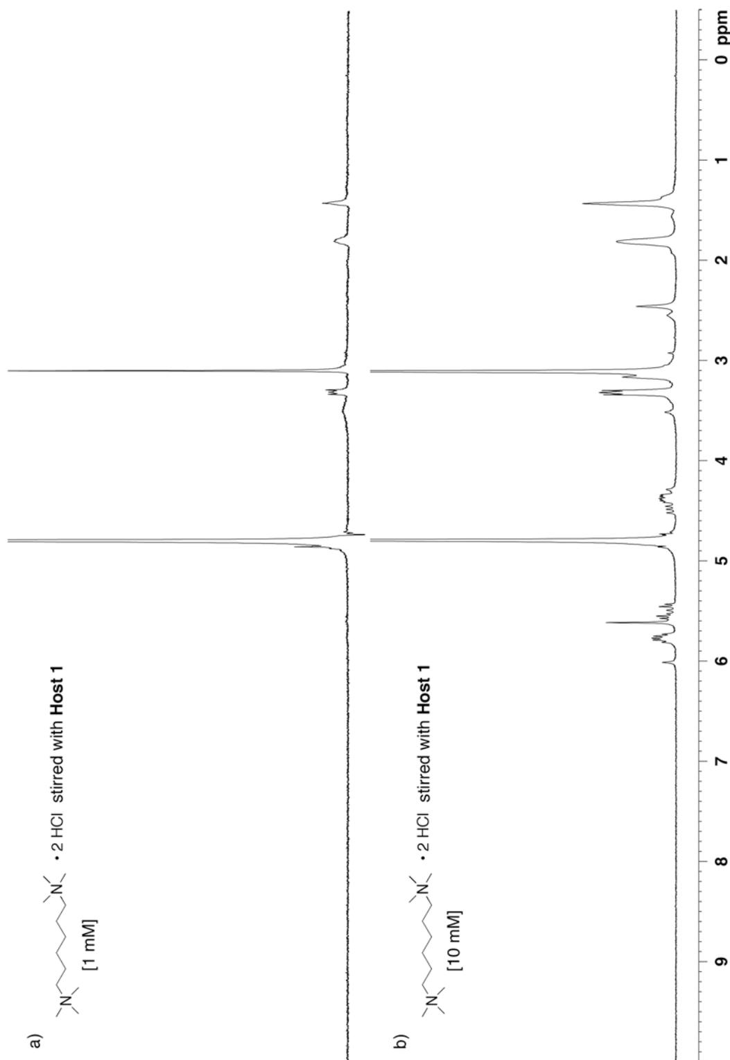
**Figure 22.**  $^1\text{H}$  NMR spectra (400 MHz,  $\text{D}_2\text{O}$ , RT) recorded for: a) a solution obtained by stirring hexamethonium chloride (1 mM) with an excess of solid **1** followed by filtration and b) a solution obtained by stirring hexamethonium chloride (10 mM) with an excess of solid **1** followed by filtration. The fact that the resonances for **1** increase higher concentration of hexamethonium chloride indicate weak binding.
