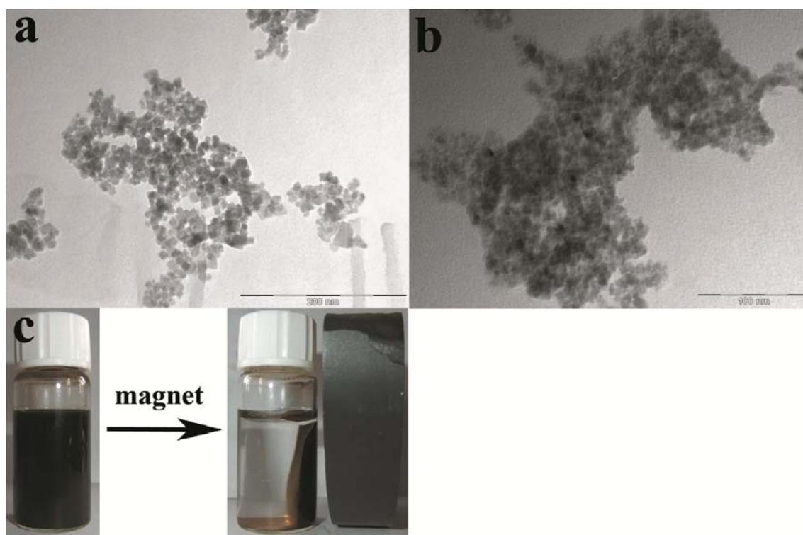
**Figure S1.** TEM images of (a)  $\text{Fe}_3\text{O}_4$  nanoparticles and (b)  $\beta$ -CD modified  $\text{Fe}_3\text{O}_4$  nanoparticles. (c) The separation process of  $\beta$ -CD modified  $\text{Fe}_3\text{O}_4$  nanoparticles from suspension under an external magnetic field.
