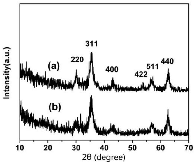
**Fig S2.** The XRD Spectra for (a) magnetic  $\text{Fe}_3\text{O}_4$  nanoparticles and (b)  $\beta$ -CD modified  $\text{Fe}_3\text{O}_4$  nanoparticles.
