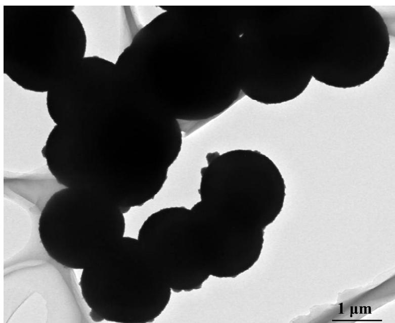
**Fig. S1** TEM images of  $V_2O_3$  solid microsphere intermediates.
