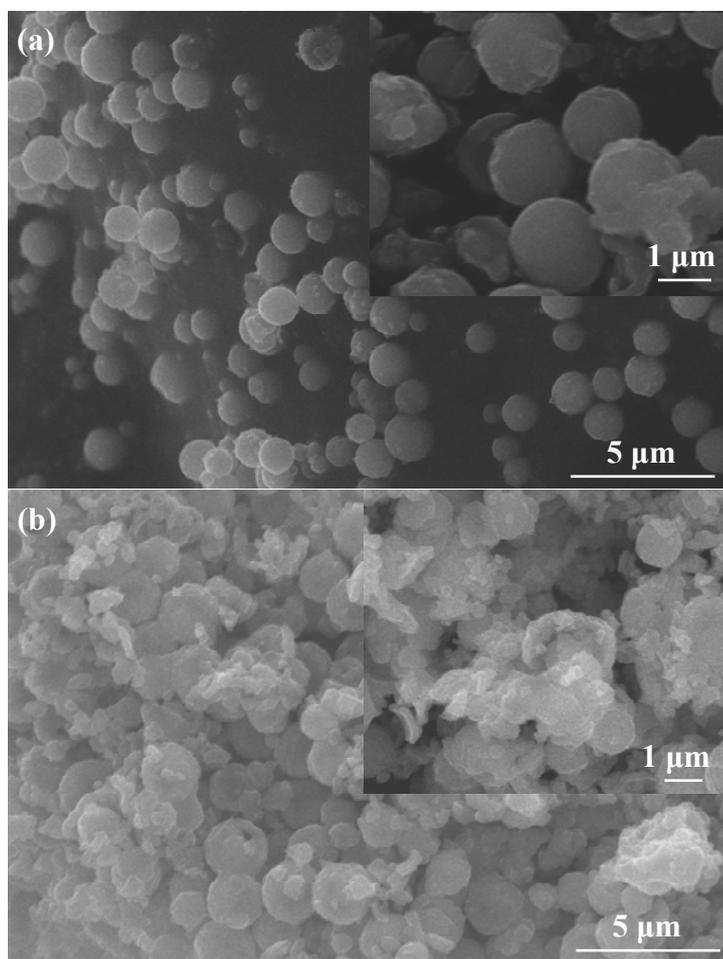
**Fig. S5** Tracking the volume changes in yolk-shell (a) and complete hollow (b)  $V_2O_5$  microspheres after 20 cycles. As shown in these SEM images, the microsphere configuration of most yolk-shell  $V_2O_5$  was preserved (Fig. S5a), while most of hollow  $V_2O_5$  microspheres collapsed (Fig. S5b), which indicates that the structure stability of yolk-shell microspheres is higher than that of completely hollow microspheres.
