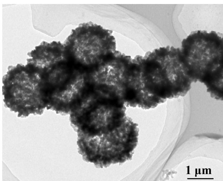
**Fig. S3** TEM image of completely hollow structured  $V_2O_5$  microspheres obtained via extending the solvothermal reaction time.
