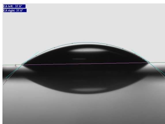
Figure S4-1. Water drop formation on cleaned gold surface (blank).
