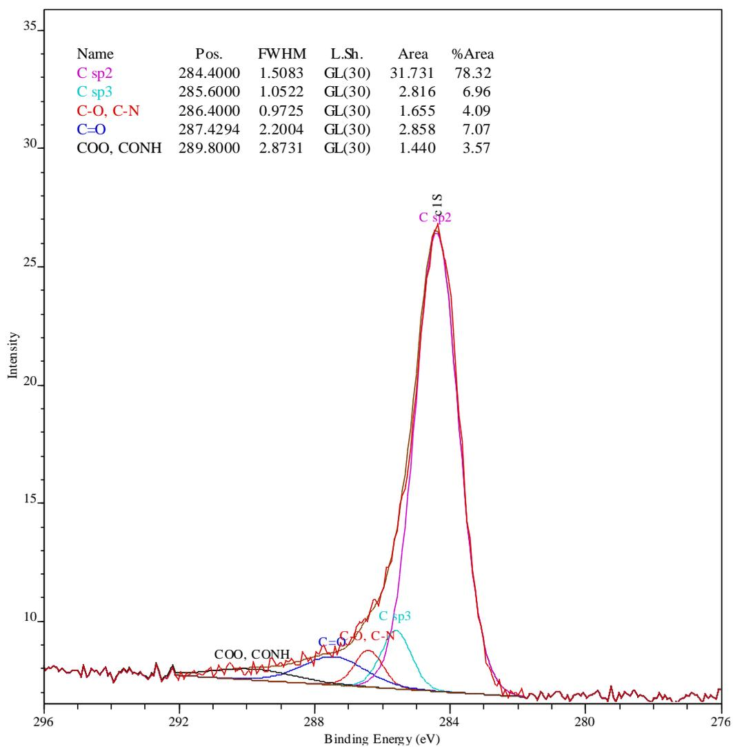
Figure S3-3. High-resolution C 1s XPS spectrum of [1•Au(111)].
