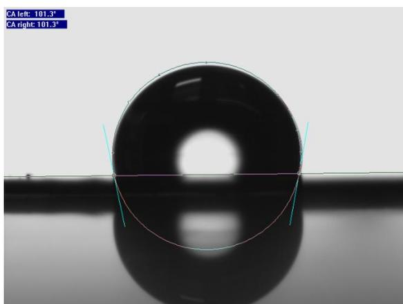
**Figure S4-4.** Water drop formation on  $CH_3(CH)_{11}SH$  modified gold surface.
