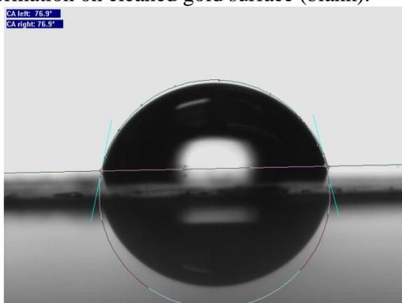
Figure S4-2. Water drop formation on 1H (C<sub>60</sub>SH) modified gold surface [1•Au(111)].
