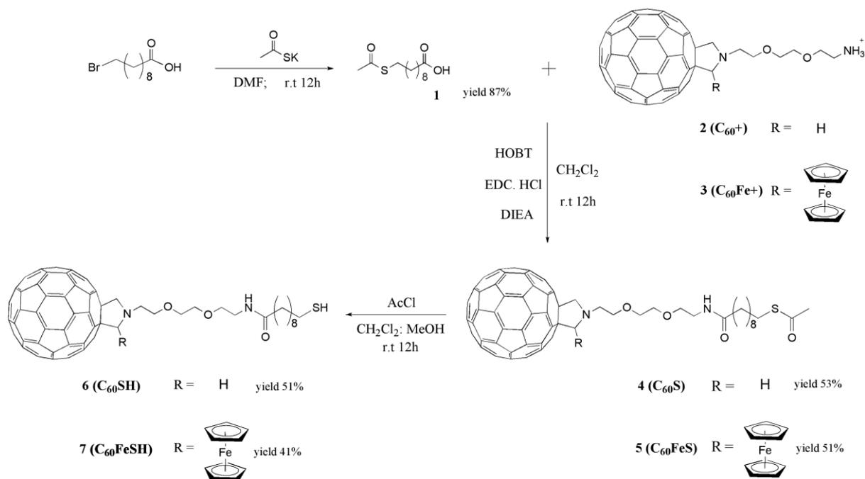
**Scheme S1.** Synthetic procedure for the production of  $\text{C}_{60}$  derivatives bearing a thiol group.
