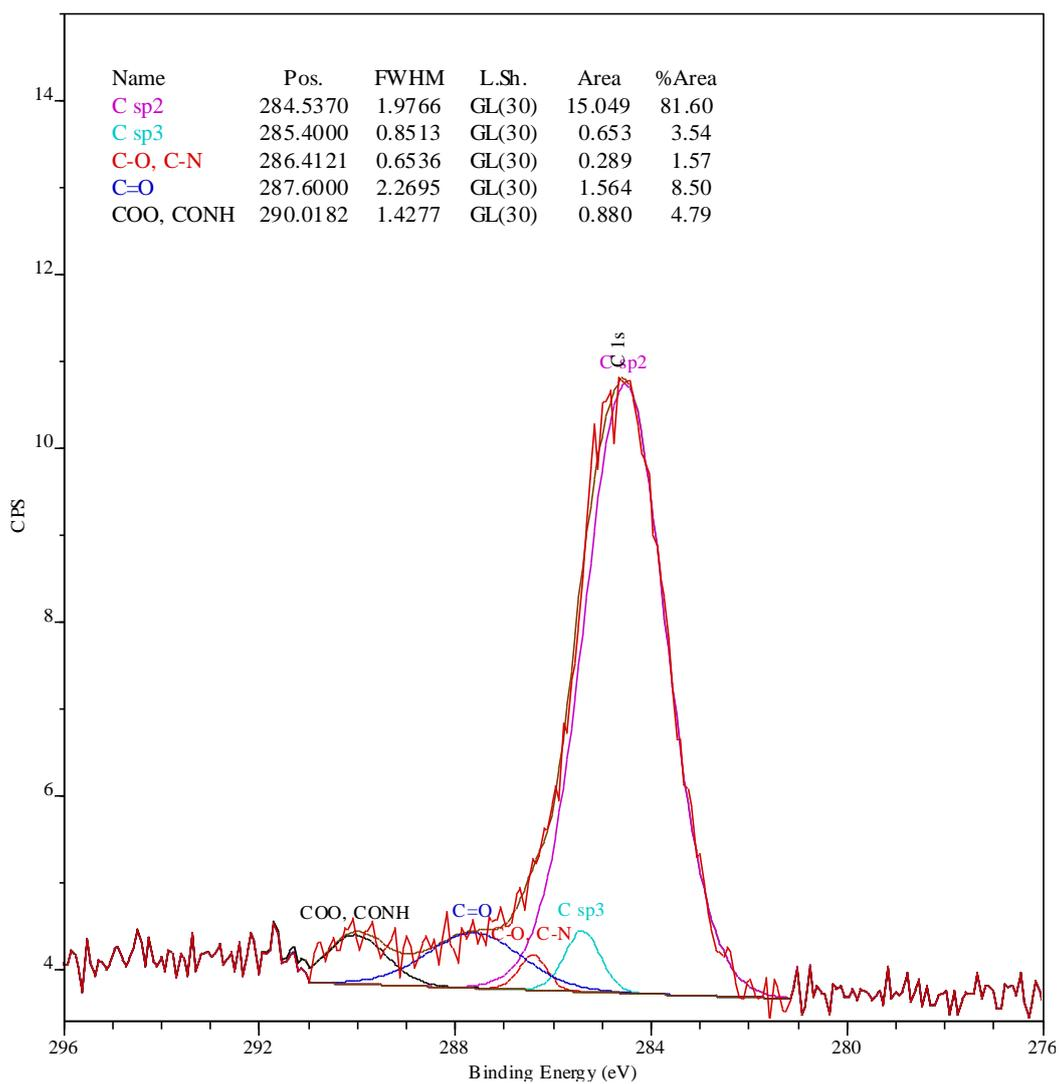
**Figure S3-4.** High-resolution C 1s XPS spectrum of [2•Au(111)].
