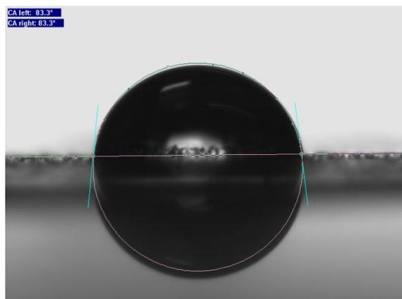
**Figure S4-3.** Water drop formation on **2H** ( $C_{60}FeSH$ ) Modified surface [**2•Au(111)**].
