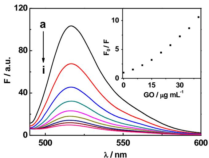
**Fig. S5.** Fluorescence spectra ( $\lambda_{\text{ex}} = 470$  nm) of FITC-labeled peptide (100 nM) in the presence of varied concentrations of GO: (a) 0, (b) 5, (c) 10, (d) 15, (e) 20, (f) 25, (g) 30, (h) 35 and (i) 40  $\mu\text{g/mL}$ . Inset shows the variation of the fluorescence intensity ratios ( $F_0/F$ ) at 516 nm versus the concentration of GO, where  $F_0$  and  $F$  are the fluorescence intensity of the FITC-labeled peptide before and after addition of GO, respectively.
