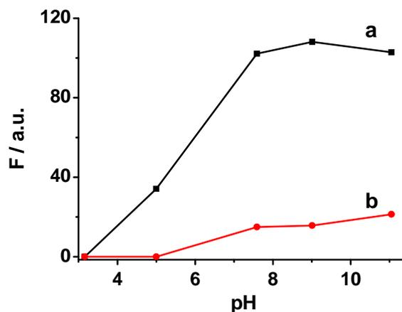
**Fig. S4.** The change in fluorescence intensity ( $\lambda_{\text{ex/em}} = 470/516$  nm) of (a) FITC (100 nM) and (b) the GO-peptide complex (in which the peptide concentration was 100 nM) at different pH values: 3.2, 5.0, 7.5, 9.0 and 11.1.
