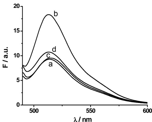
**Fig. S9.** Fluorescence spectra of different reaction systems. (a): the GO-peptide complex (100 nM) in the TCNB buffer (control); (b): (a) + MMP2 (5 nM); (c): (a) + 1,10-phenanthroline (10  $\mu\text{M}$ ); (d): (b) + 1,10-phenanthroline (10  $\mu\text{M}$ ).  $\lambda_{\text{ex}} = 470$  nm.
