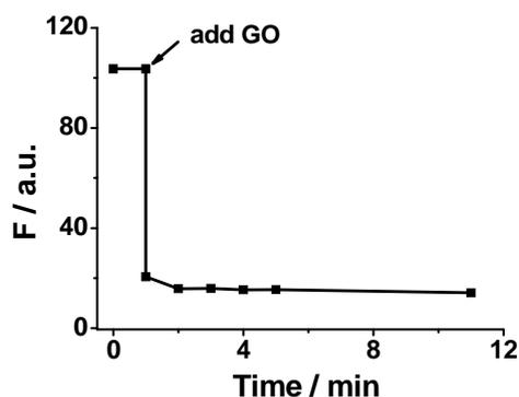
**Fig. S6.** Fluorescence quenching of the FITC-labeled peptide (100 nM) in TCNB buffer with 30 µg/mL GO as a function of incubation time at room temperature.  $\lambda_{\text{ex/em}} = 470/516$  nm.
