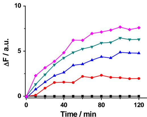
**Fig. S8.** The effect of reaction time on the fluorescence change of the GO-peptide complex reacting with varied concentrations of MMP2 (from bottom to top: 0.0, 0.5, 1.0, 1.5, and 2.0 nM) in TCNB buffer at 37 °C.  $\lambda_{\text{ex/em}} = 470/516$  nm.
