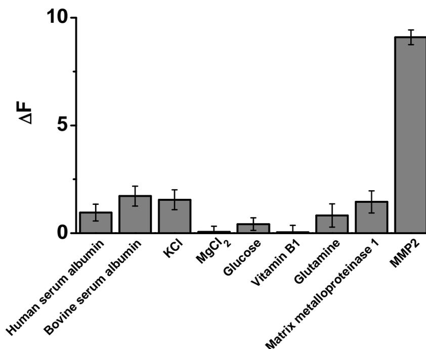
**Fig. S10.** Fluorescence responses of the GO-peptide complex (100 nM) to various substances: human serum albumin (100 nM), bovine serum albumin (100 nM), KCl (150 mM), MgCl<sub>2</sub> (2.5 mM), glucose (10 mM), vitamin B1 (1 mM), glutamine (1 mM), matrix metalloproteinase 1 (5 nM), or MMP2 (5 nM).  $\Delta F$  is the difference of the fluorescence intensity of the GO-peptide complex in the presence and absence of a substance.
