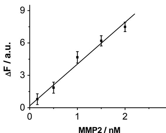
**Fig. S7.** Fluorescence intensity change ( $\Delta F$ ) of the GO-peptide as a function of MMP2 concentration.  $\Delta F$  is the difference of fluorescence intensity of the GO-peptide complex in the presence and absence of MMP2. The data shown here represent the means and standard deviations of three independent experiments.  $\lambda_{\text{ex/em}} = 470/516$  nm.
