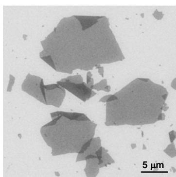
**Fig. S1.** The scanning electron microscopy image of GO.
