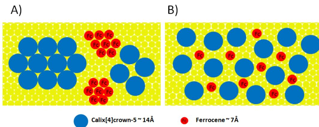
**Figure S3: The schematic drawing of the mixed SAM of the receptor 1 and the guest 3 on the surface of the gold electrode**
