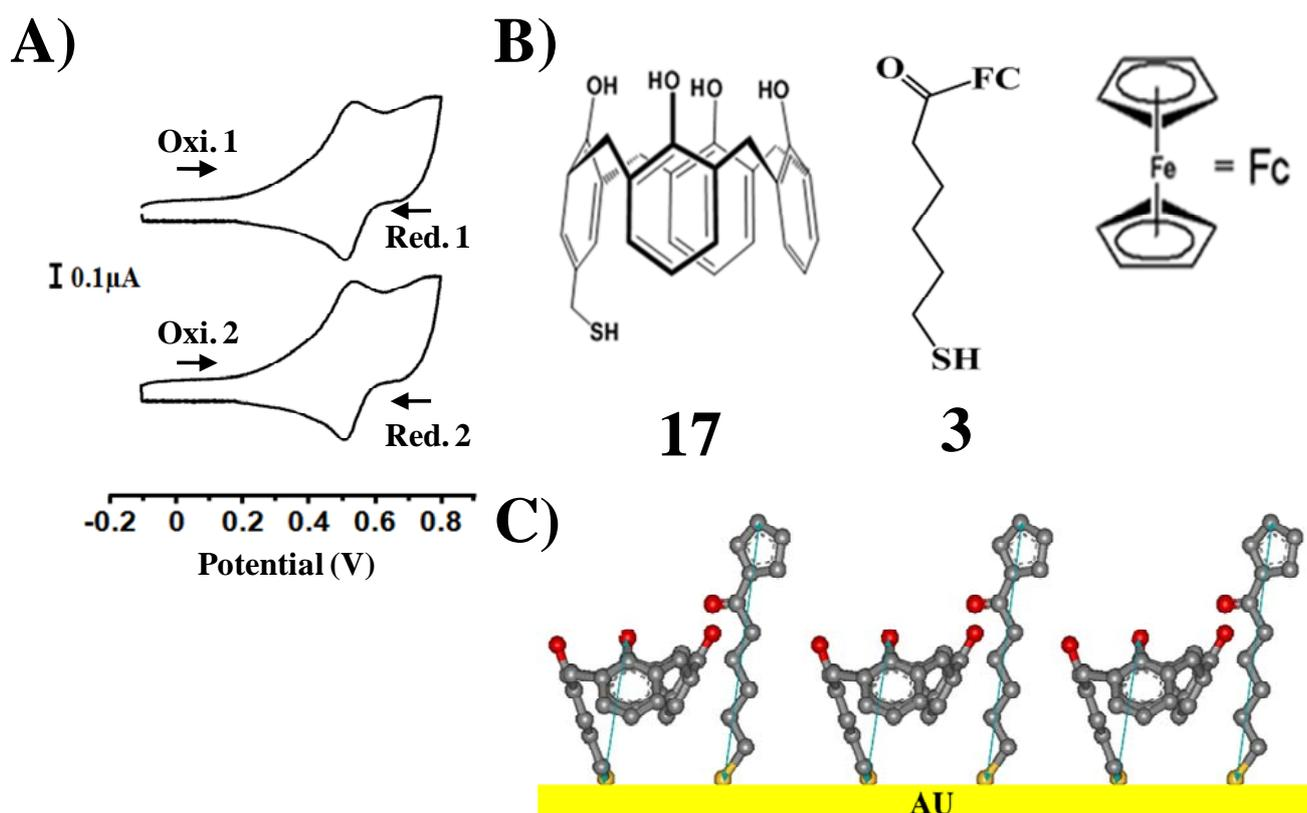
**Figure S5: Interaction of the receptor **17** and guest **3** in the mixed SAM on the gold surface.** A) First and Second consecutive cyclic voltammograms of the gold electrode modified with the mixed-SAM of the receptor **17** and guest **3**. B) The monothiolated calix[4]arene receptor **17** and guest **3**, C) Mixed self-assembled monolayer of the monothiolated calix[4]arene receptor **17** and guest **3**.
