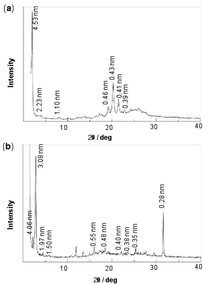
**Figure S5.** X-ray diffraction patterns of **2** (a) and a mixture of **4** with **5** plus NaCl (b) in film state.
