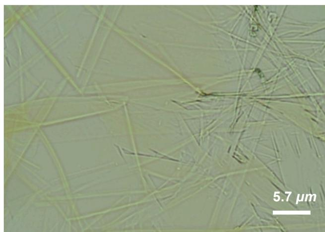
**Figure S11.** The optical image of compounds obtained by reaction of sodium lauryl sulfate with **1** by treatment of excess HCl in THF solution.
