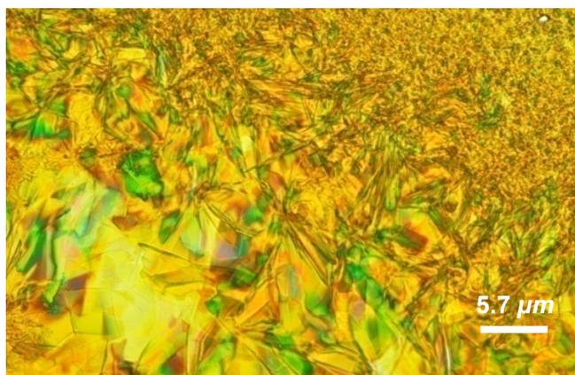
**Figure S9.** The optical image of solid mixture obtained by reaction of azopyridine **1** with DBSA **3** in a THF solution without addition of HCl.
