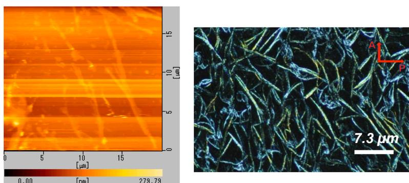
**Figure S7.** AFM (left) and POM (right) images of nanofibers fabricated with **2**. A, analyzer; P, polarizer.
