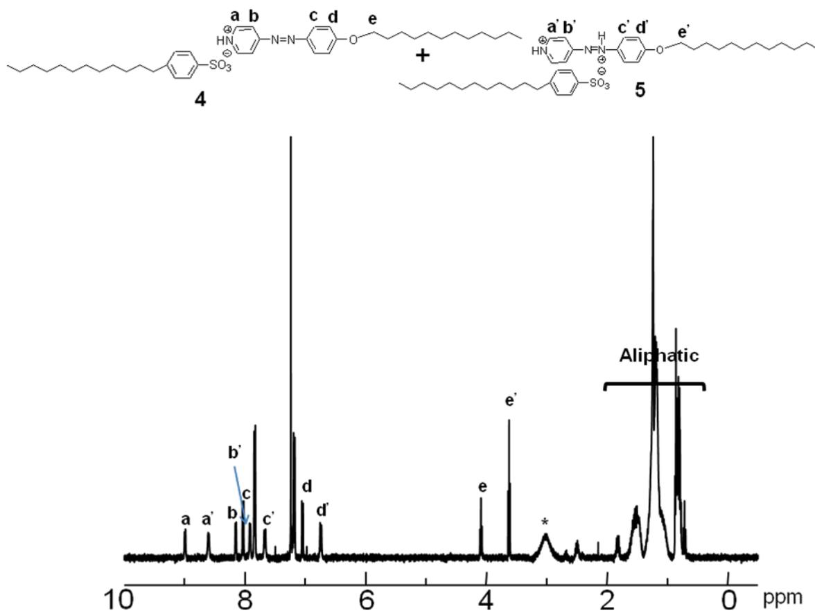
**Figure S4.**  $^1\text{H}$  NMR spectrum and its assignment of a mixture of **4** with **5** in  $\text{CDCl}_3$ .
