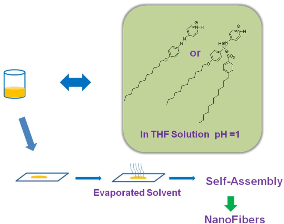
**Figure S6.** Illustration of the fabrication processes of organic nanofibers.
