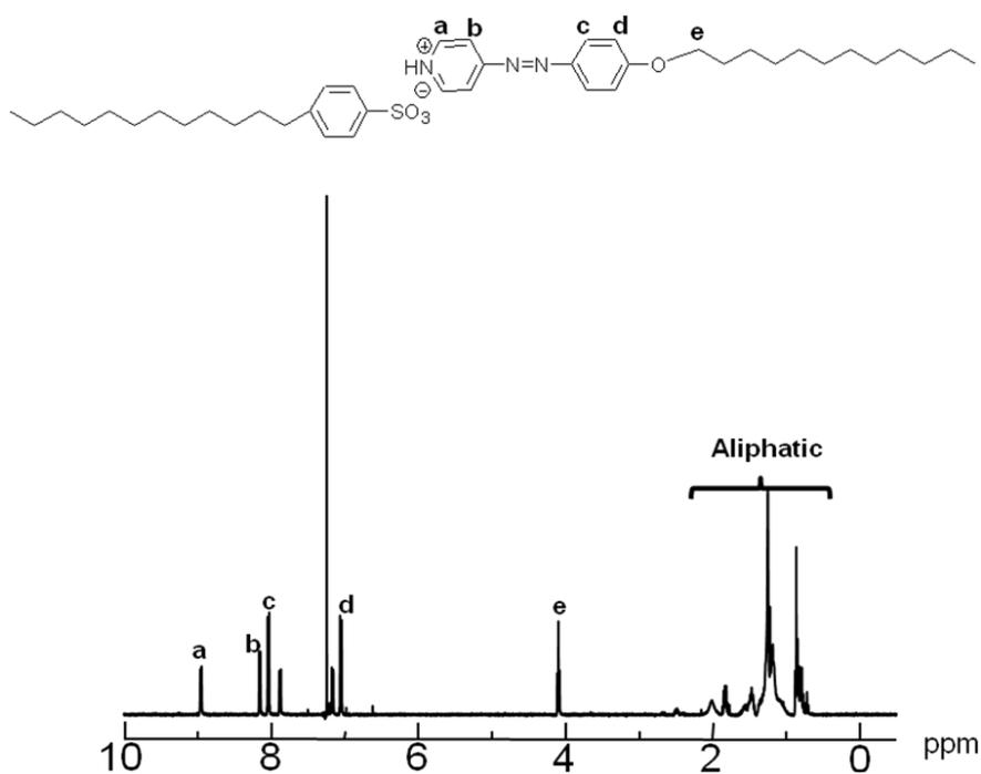
**Figure S3.** <sup>1</sup>H NMR spectrum and its assignment of compound of **4** in CDCl<sub>3</sub>.
