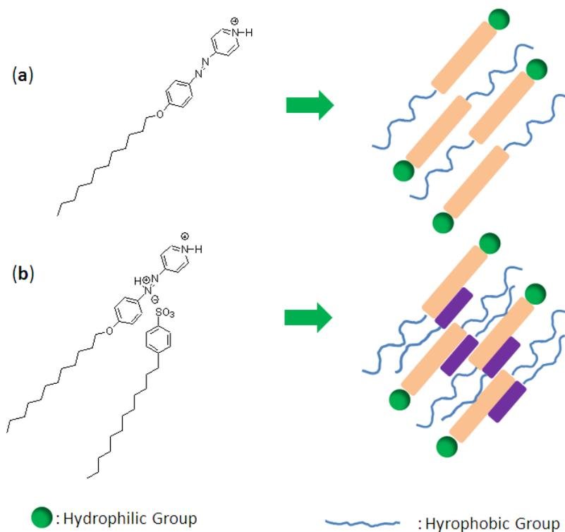
**Figure S13.** Possible schemes of the fabricated organic nanofibers and their hybrids. (a) nanofibers, (b) hybrid nanofibers.
