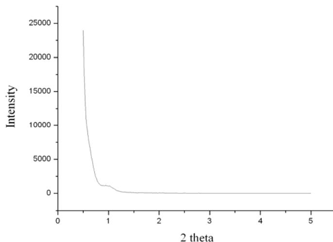
**Figure S6.** Small angle XRD pattern for Pd@SBA-15<sup>©</sup>.
