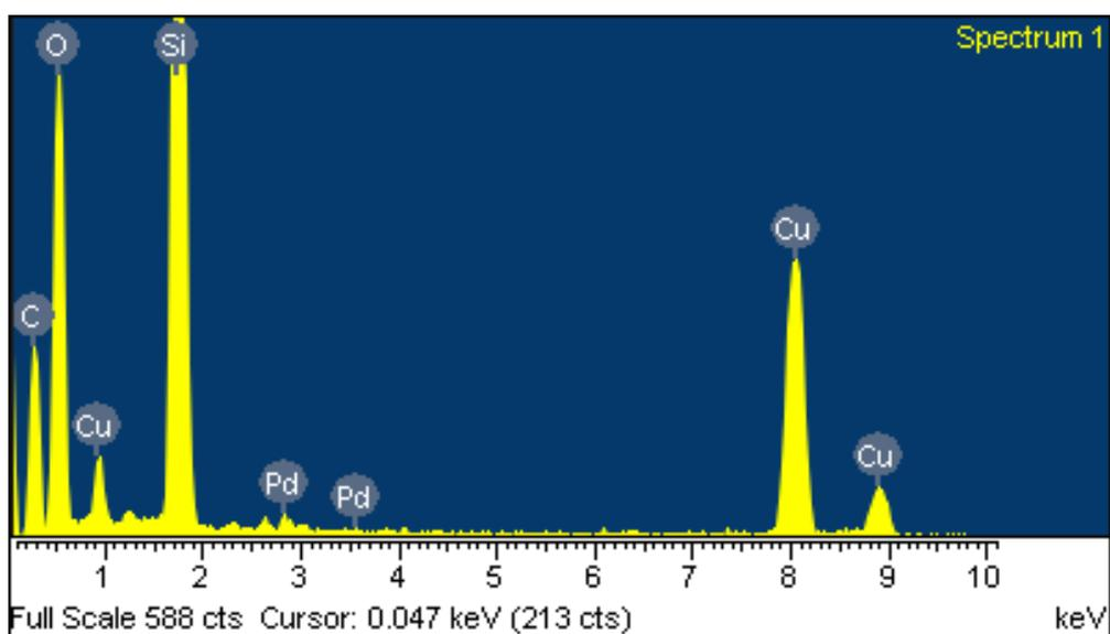
**Figure S2.** EDS spectrum of Pd@SBA-15<sup>©</sup>.
