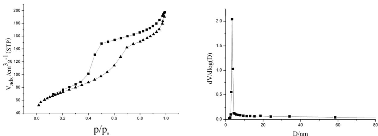
**Figure S5.** Nitrogen adsorption isotherms at 77 K (left) and pore-size distribution curves (right) of Pd@SBA-15<sup>®</sup>.
