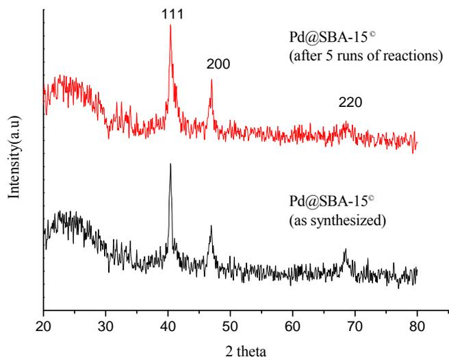
**Figure S3.** Wide angle XRD patterns for Pd@SBA-15<sup>®</sup> catalysts recorded before and after catalytic reaction.
