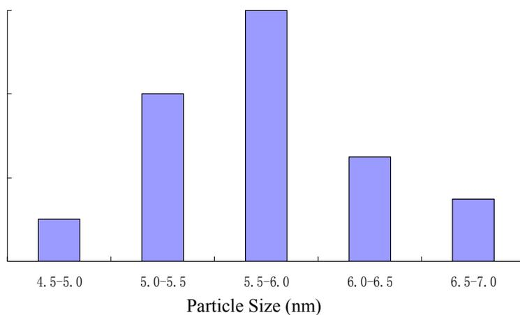
**Figure S4.** Pd particle size distribution of Pd@SBA-15<sup>®</sup> as measured with TEM.
