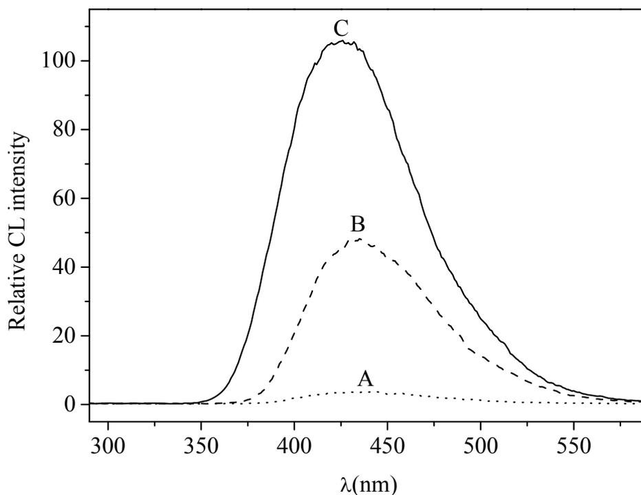
**Figure S4.** The CL spectra of 100  $\mu$ M hydrogen peroxide–100  $\mu$ M luminol reaction product catalyzed by CoFe<sub>2</sub>O<sub>4</sub> or HRP; (A): luminol–hydrogen peroxide; (B): luminol–hydrogen peroxide–0.1  $\mu$ M HRP; (C): luminol–hydrogen peroxide–8 mg/L CoFe<sub>2</sub>O<sub>4</sub>.
