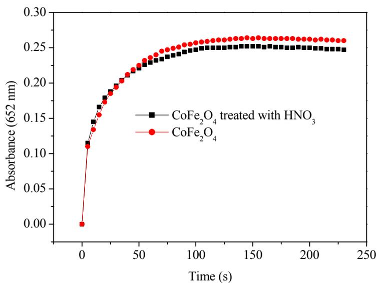
**Figure S10.** Illustration that CoFe<sub>2</sub>O<sub>4</sub> activity does not result from metal leaching. The as-prepared CoFe<sub>2</sub>O<sub>4</sub> nanoparticle was treated with (square) and without nitric acid (circle). CoFe<sub>2</sub>O<sub>4</sub> concentration: 8 mg/L, TMB: 0.4 mM; H<sub>2</sub>O<sub>2</sub>: 0.1 mM; pH=6.0.
