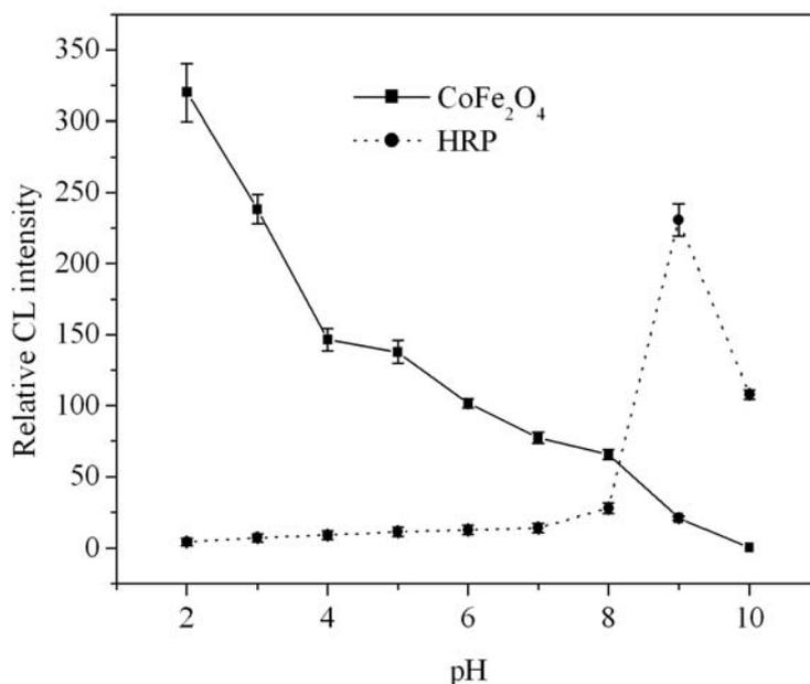
**Figure S5.** Effect of pH on catalytic activity of CoFe<sub>2</sub>O<sub>4</sub> and HRP. Experimental conditions: 1  $\mu$ M luminol in 0.1 M buffer solution of Na<sub>2</sub>CO<sub>3</sub>-NaHCO<sub>3</sub> (pH 10.15), 10  $\mu$ M hydrogen peroxide, 8 mg/L CoFe<sub>2</sub>O<sub>4</sub> or 0.1  $\mu$ M HRP at 25 °C. Error bars represent one standard deviation for five measurements.
