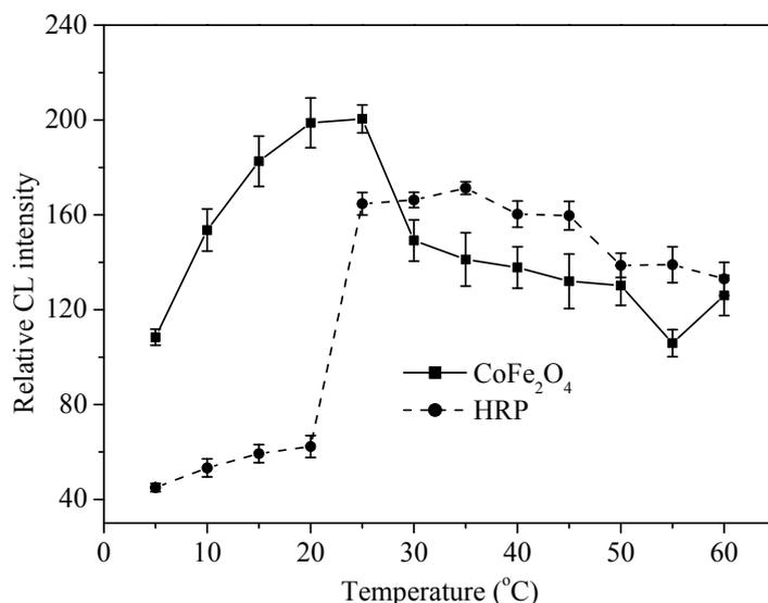
**Figure S6.** Effect of temperature on catalytic activity of CoFe<sub>2</sub>O<sub>4</sub> and HRP. Experimental conditions: 1  $\mu$ M luminol in 0.1 M buffer solution of Na<sub>2</sub>CO<sub>3</sub>-NaHCO<sub>3</sub> (pH 10.15), 10  $\mu$ M hydrogen peroxide, 8 mg/L CoFe<sub>2</sub>O<sub>4</sub> (pH 6.0) or 0.1  $\mu$ M HRP (pH 8.6). Error bars represent one standard deviation for five measurements.
