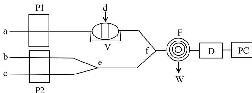
**Figure S3.** Schematic for flow-injection analysis system. (P1) and (P2) Peristaltic pumps; (a) Carrier; (d)  $\text{CoFe}_2\text{O}_4$  or HRP; (V) Injection valve; (e) and (f) Tee; (b) Hydrogen peroxide; (c) Luminol; (F) Flow cell; (W) Waste liquid; (D) Detector; (PC) Personal computer.
