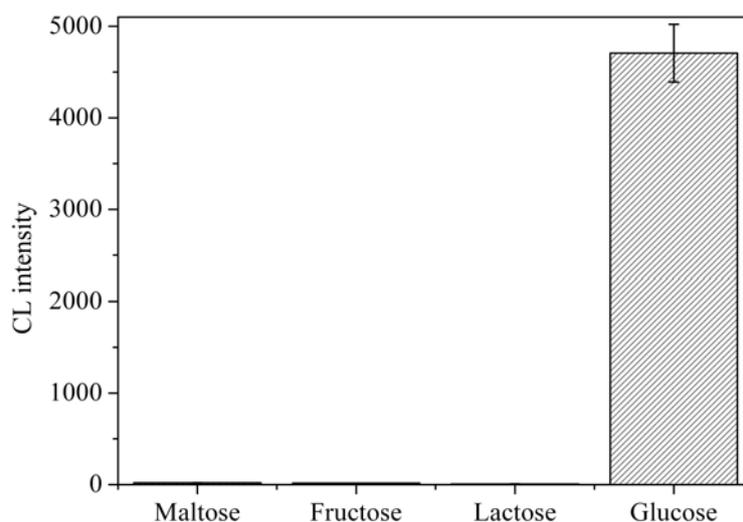
**Figure S11.** Selectivity analysis for glucose detection by monitoring the relative CL intensity. The analyte concentrations were as follows: 10 mM fructose, 10 mM lactose, 10 mM maltose, and 10  $\mu$ M glucose. The error bars represent the standard deviation of five measurements.
