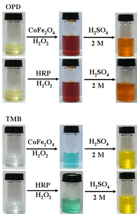
**Figure S9.** Images of oxidation color reaction of OPD or TMB by H<sub>2</sub>O<sub>2</sub> after catalyzing by CoFe<sub>2</sub>O<sub>4</sub> or HRP, and subsequently being quenched by H<sub>2</sub>SO<sub>4</sub>.
