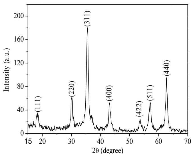
**Figure S1.** XRD patterns of  $\text{CoFe}_2\text{O}_4$
