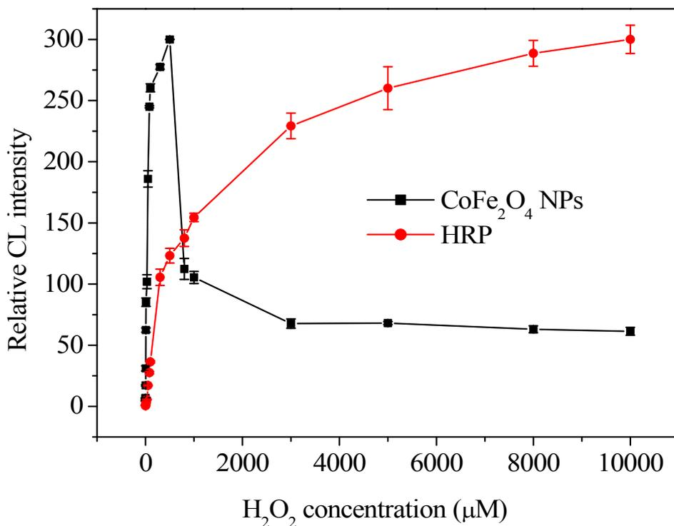
**Figure S7.** Effect of the hydrogen peroxide concentration on catalytic activity of CoFe<sub>2</sub>O<sub>4</sub> and HRP. Experimental conditions: 1 μM luminol in 0.1 M buffer solution of Na<sub>2</sub>CO<sub>3</sub>-NaHCO<sub>3</sub> (pH 10.15), 8 mg/L CoFe<sub>2</sub>O<sub>4</sub> (pH 6.0) or 0.1 μM HRP (pH 8.6), the temperature is 25 °C. Error bars represent one standard deviation for three measurements.
