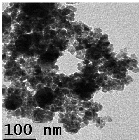
**Figure S2.** TEM image of  $\text{CoFe}_2\text{O}_4$
